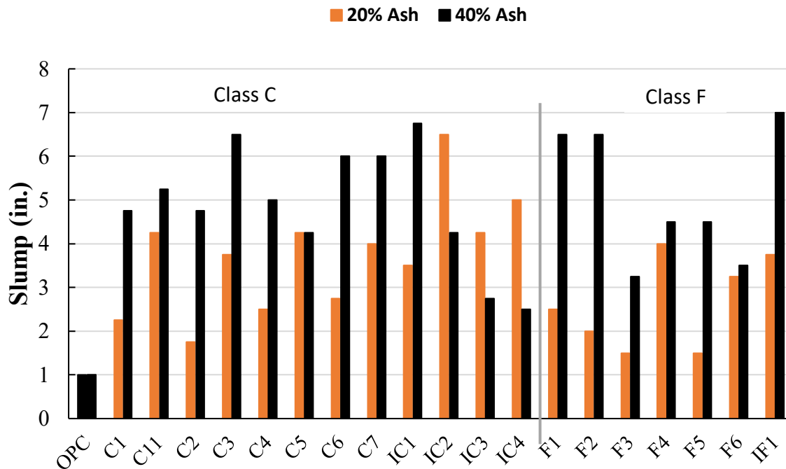
Figure 1. Graph. Comparison of slumps measured for each fly ash mixture at 20% and 40% replacement levels.
