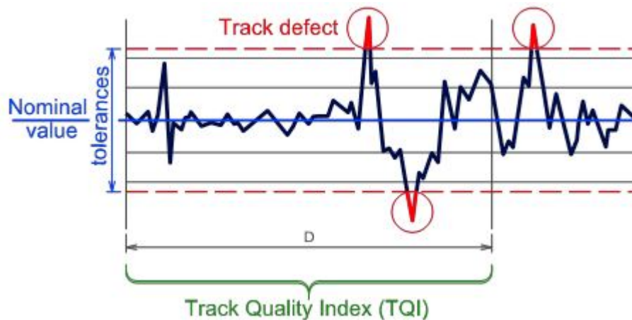
Figure 2: Track quality indices, tolerances and defects (Ciobanu 2016)
