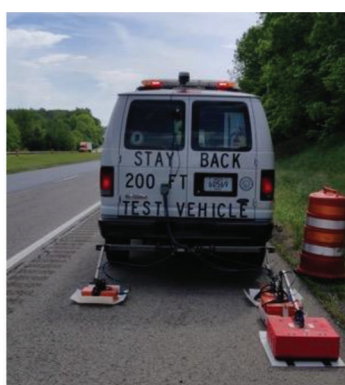
(a) Test vehicle with GPR antennas attached.
