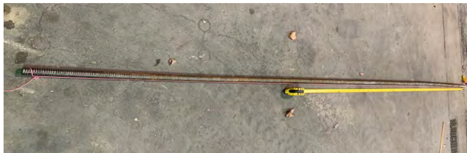
Figure 5.8 PT bar buckling
