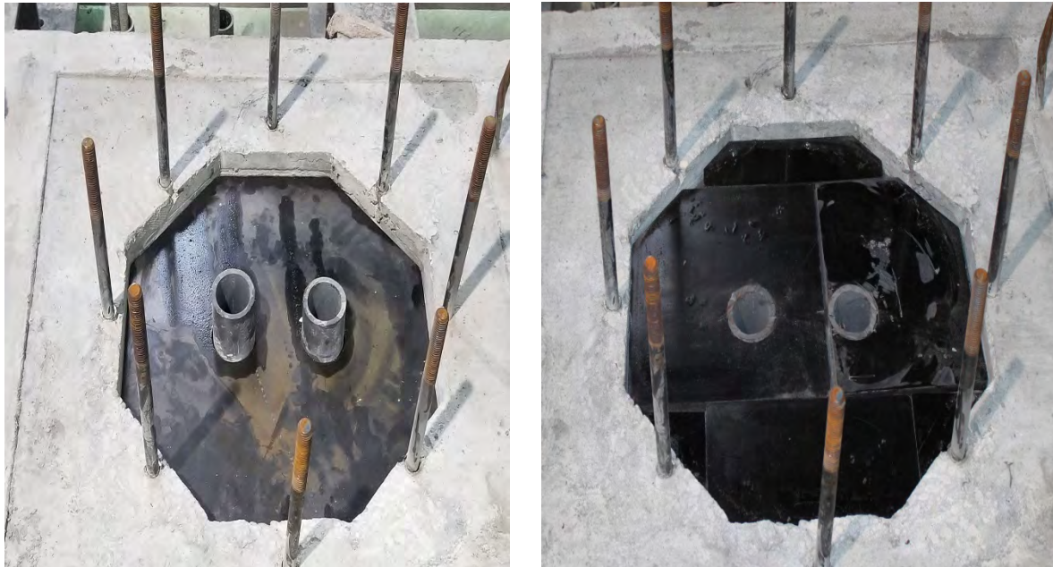
Figure 3.13 1/2" (12.7 mm) thick steel plate and 1/2" (12.7 mm) polyurethane plate on the footing recess
