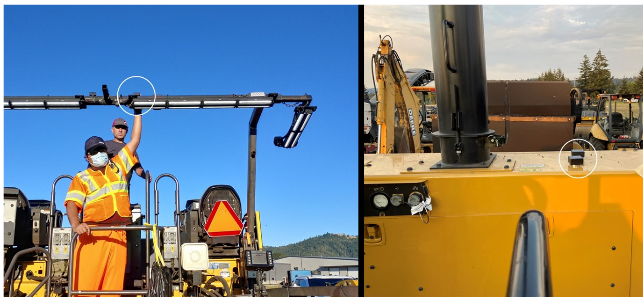
Figure 2.8: GPS sensor location on the paver light bar (left) and on top of paver (right)
