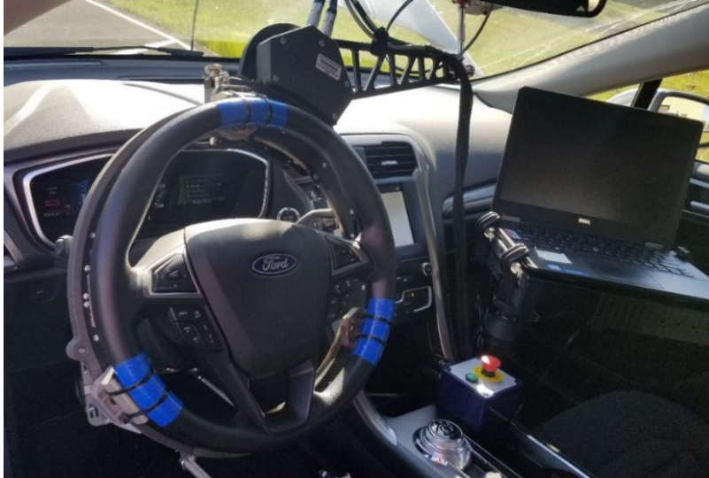
Figure 2-3. Example steering robot installation
