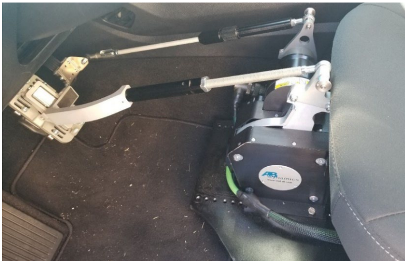
Figure 2-4. Example accelerator robot installation
