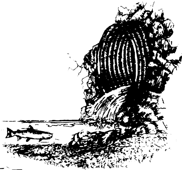
No resting pool below culvert
