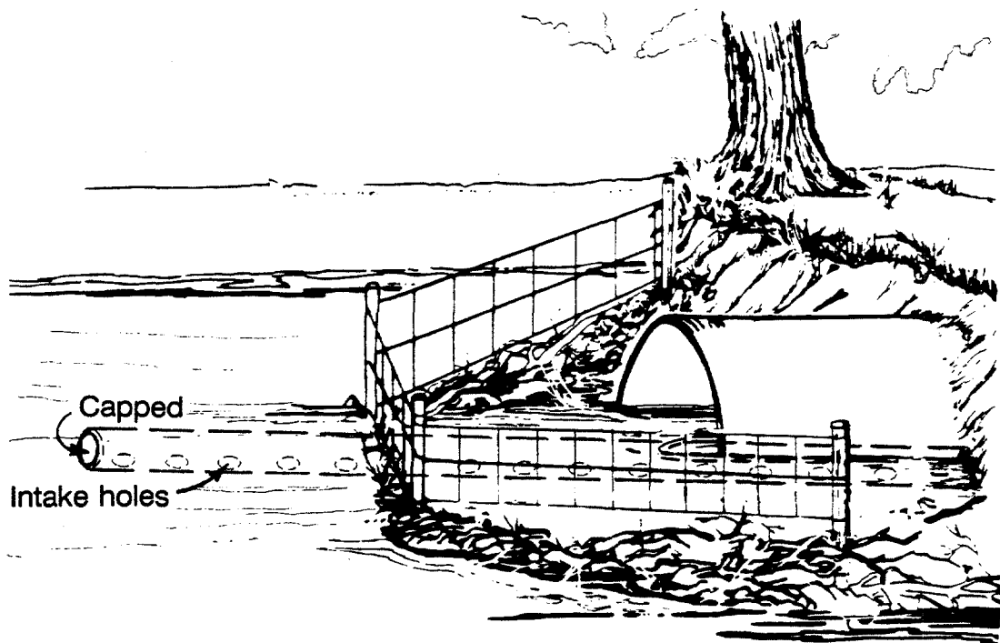
Figure B.24.1. The perforated pipe method.
