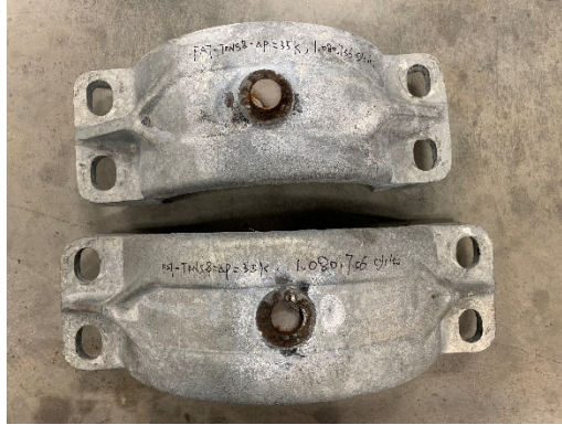
Figure 4.26: Failure of FAT-TENS8 Tested at 5.8 ksi
