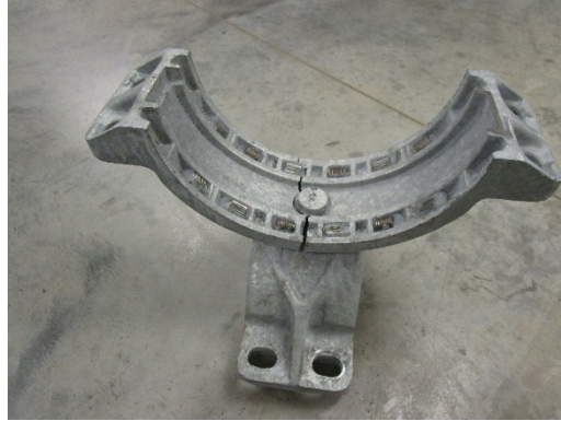
Figure 4.20: Failure of FAT-TENS4 Tested at 5.8 ksi
