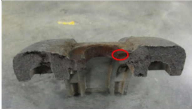
(a) Fracture Surface of FAT-TENS(USED)1
