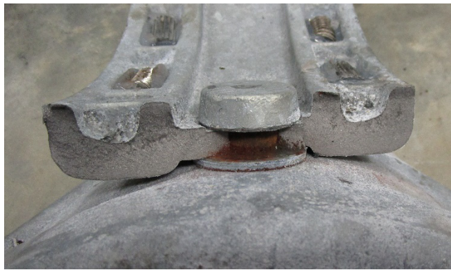
Figure 4.29: Corrosion Products on Failure Surface of FAT-TENS4
