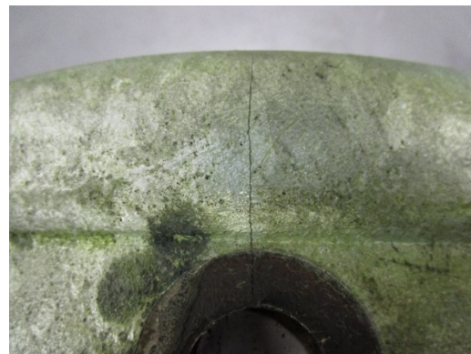
(b) Crack on the 10-in. Coupler
