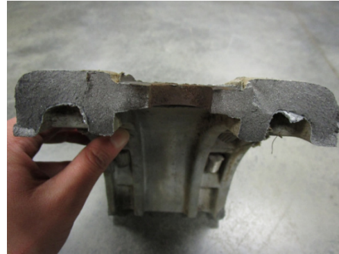
(b) Failure Surface of FAT-TENS(USED)2
