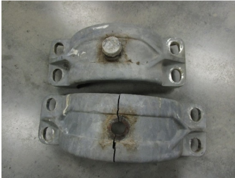
(a) Failure of FAT-TENS(USED)2
