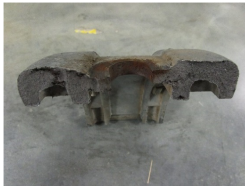
Figure 4.5: Failure Surface of FAT-TENS(USED)1
