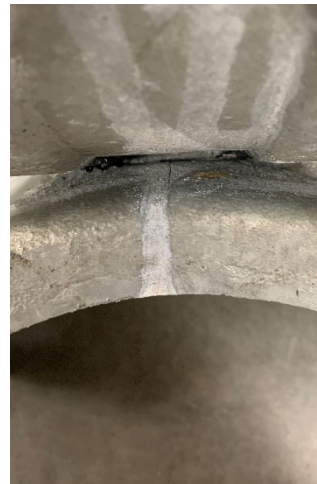
(b) Crack on the Other Side Propagated to the Edge
