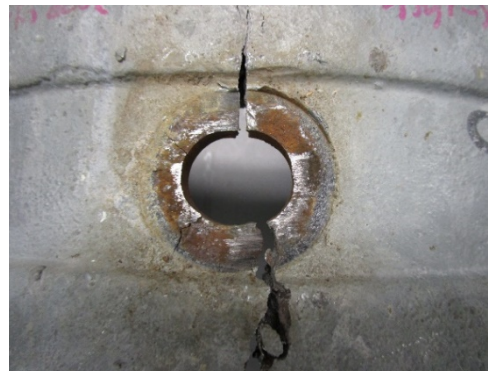
(b) Cracked 10-in. Coupler
