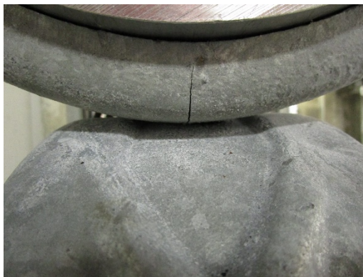
(a) Crack at 7,214,300 Cycles
