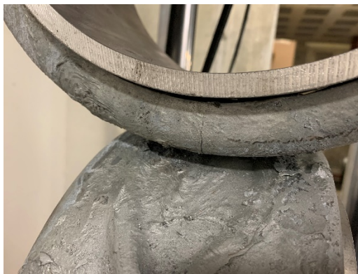
(a) Crack at 632,420 Cycles
