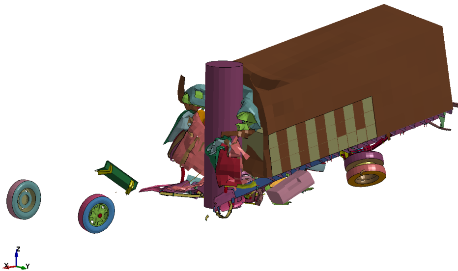
Figure 3.6: F800 and semi-rigid column at 0.174 seconds after impact
