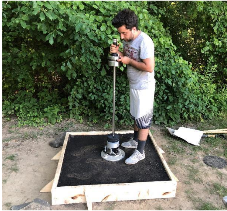
Figure 4: Field Scale Model Evaluation (FSME) Testing System
