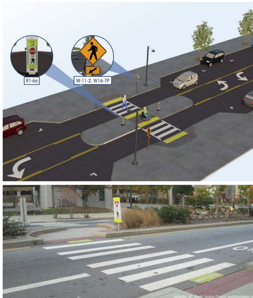
Figure D.6 Pedestrian refuge island (FHWA, 2018f).
