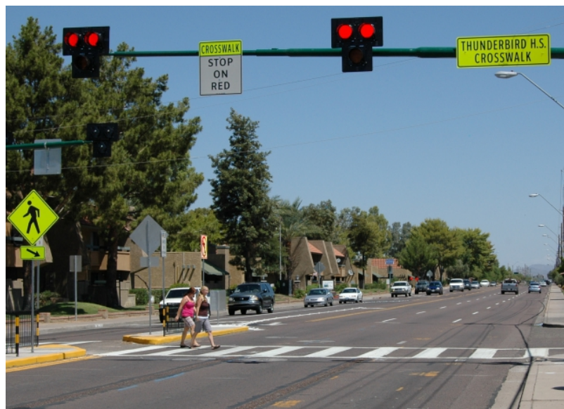
Figure D.2b Example of Pedestrian Hybrid Beacon in Phoenix AZ (pedbikeimages.org/Mike Cynecki).
