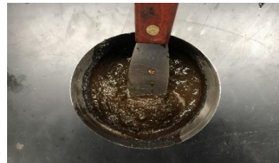
(h) Microsurfacing Mixing Process
