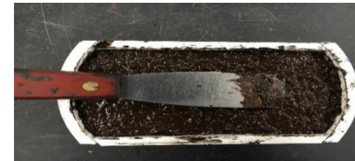
(i) Pouring &amp; Spreading Microsurfacing Mix
