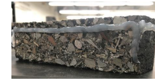
(a) Silicon Sealant Application
