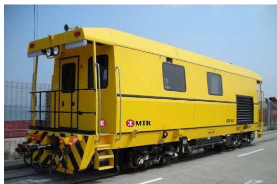
Figure 2.6. Ultrasonic Test Done by Vehicle (Railway Technology, 2013)
