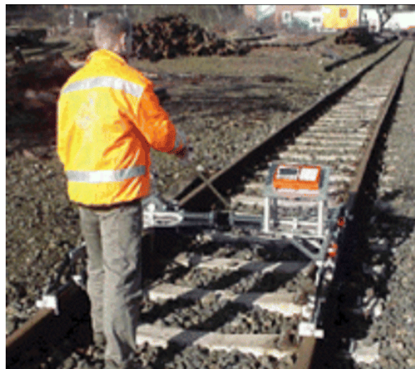
Figure 2.5. Ultrasonic Test Conducted by Hand (Zarembski and Palese, 2005)
