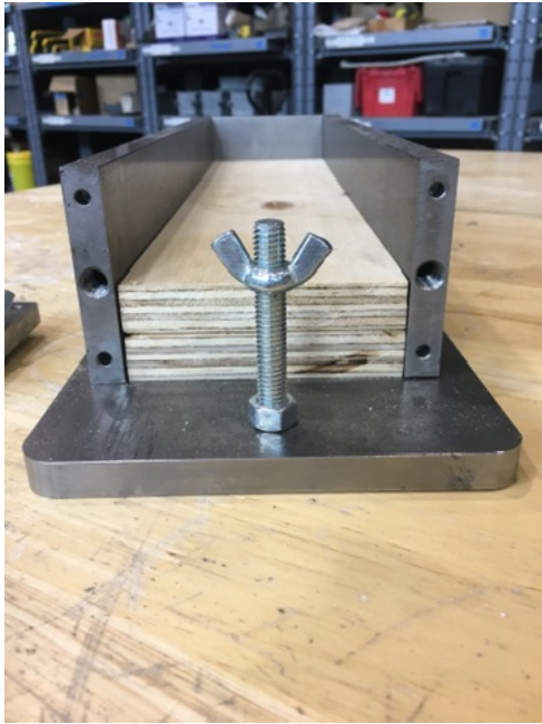
Figure 4.1 (a) & (b): Substrate casting setup
