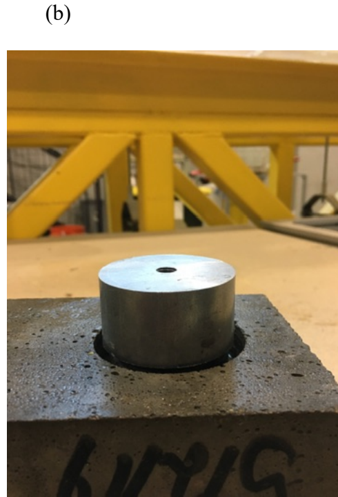
Figure 4.5: Preparation of a specimen for ASTM C1583 by core drilling
