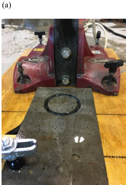
Figure 4.5: Preparation of a specimen for ASTM C1583 by core drilling
