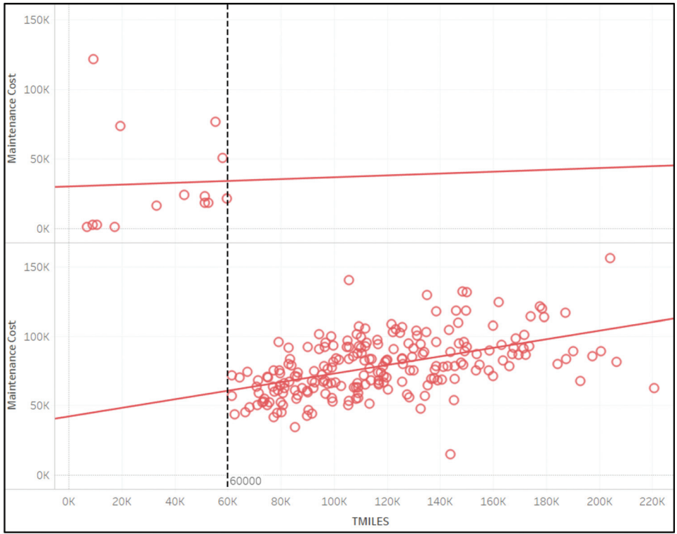
Figure 6.14 Analysis of maintenance cost vs. miles driven of single axle INDOT dump trucks.
