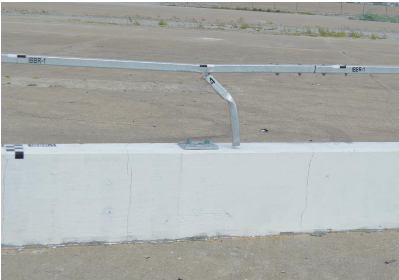
Figure 32. Back Side System Damage, Test No. IBBR-1
