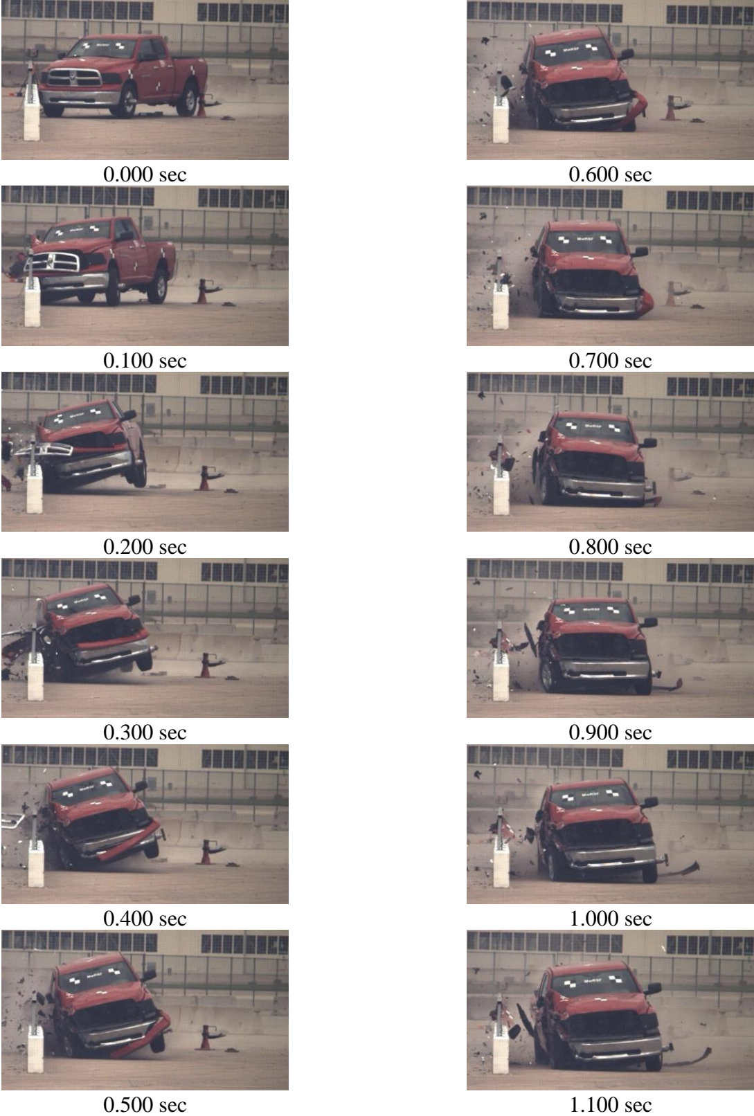
Figure 27. Additional Sequential Photographs, Test No. IBBR-1
