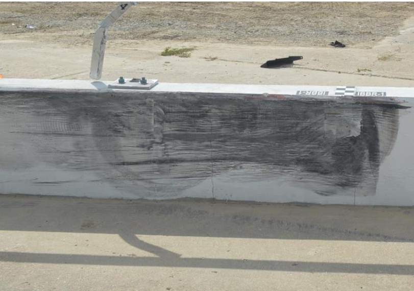
Figure 31. Front Side System Damage, Test No. IBBR-1
