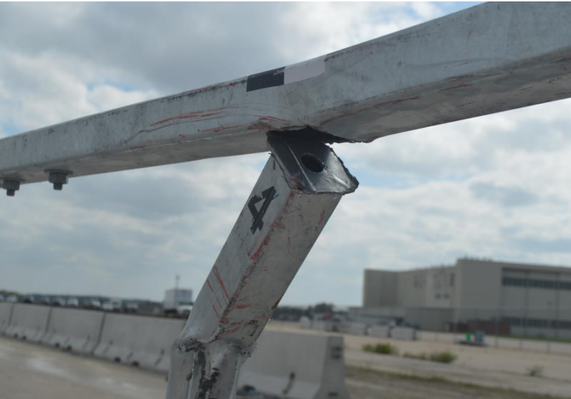
Figure 33. Post No. 4 Damage, Test No. IBBR-1
