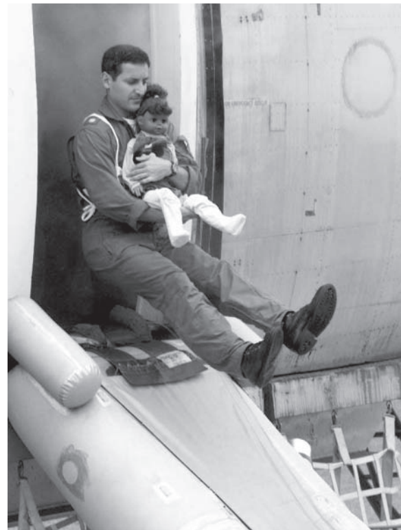
Figure 12. Infant carrier hold 24-month dummy vertically and jumps onto slide.
