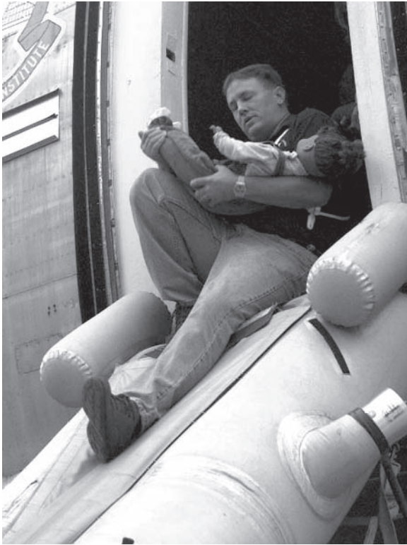
Figure 13. Infant carrier with 24-month dummy sits on slide to board.
