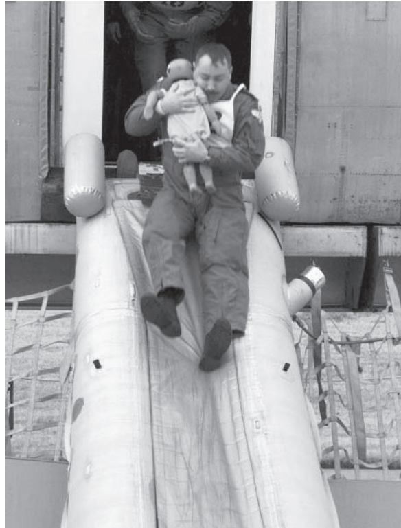
Figure 10. Infant carrier hold 6-month dummy vertically and jumps onto slide.
