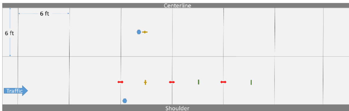
Legend ↔ Joint Opening Sensor — Dynamic Strain Gauge* + Vibrating Wire Strain Gauge* ● Temperature Tree *Strain gauges placed at top and bottom of concrete at each location shown
