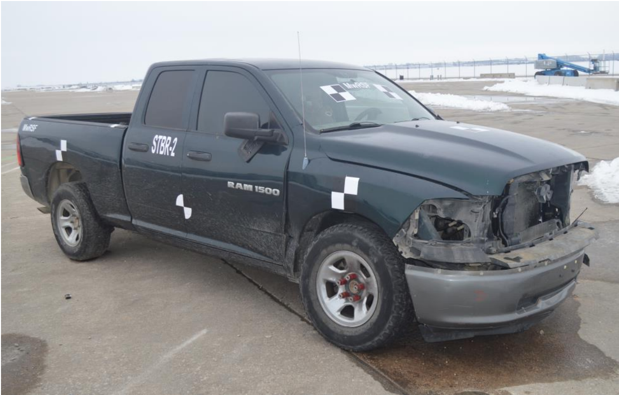
Figure 231. Vehicle Damage, Right-Corner Views, Test No. STBR-2
