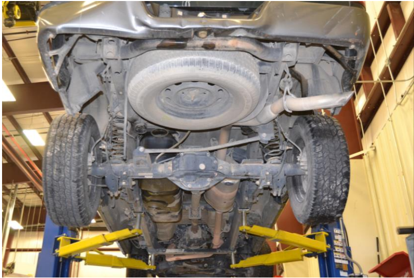
Figure 233. Vehicle Damage, Floor Pan and Undercarriage, Test No. STBR-2
