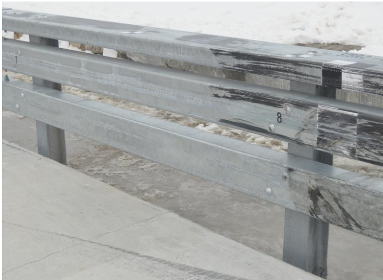
Figure 219. System Damage, Rail Span Between Posts Nos. 7 and 8, Test No. STBR-2
