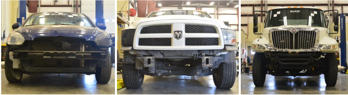
Figure 38. MASH Small Car, Pickup Truck, and SUT Front Bumper Rigid Bodies
