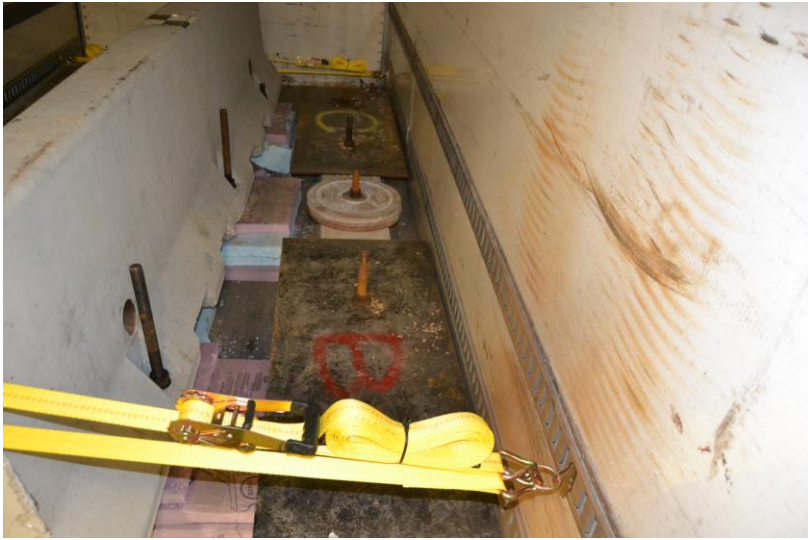
Figure 123. Nylon Straps and Ballast Installation, Test No. STBR-1
