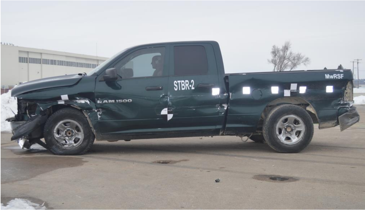
Figure 230. Vehicle Damage, Right and Left Views, Test No. STBR-2
