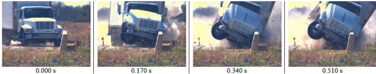
Figure 23. 36-in. (914-mm) Tall, Single-Slope, Traffic Rail Bridge Rail under MASH TL-4 Impact Conditions [38]
