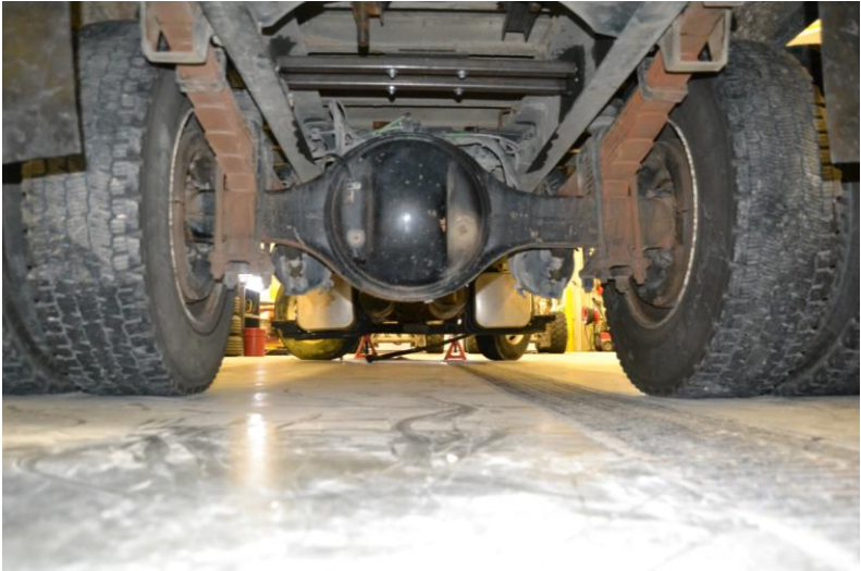
Figure 178. Vehicle Damage, Floor Pan and Undercarriage, Test No. STBR-1
