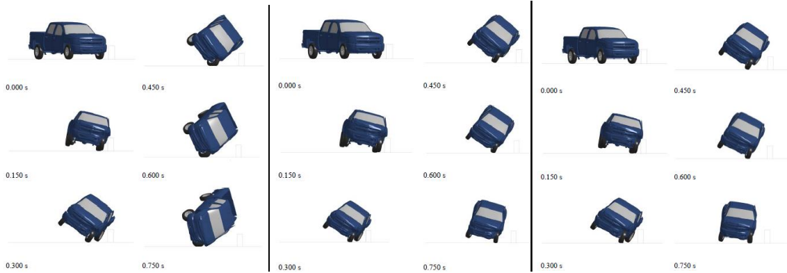
Figure 20. FE Simulations of MASH Pickup Truck Impacting a 27-in. (left), 28-in. (middle), and 29-in. (right) Tall Rigid Barriers [36]
