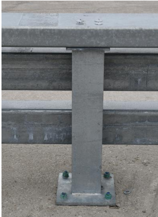
Figure 156. Test Installation Photographs, Side-Mounted and Top-Mounted Posts, Test No. STBR-1
