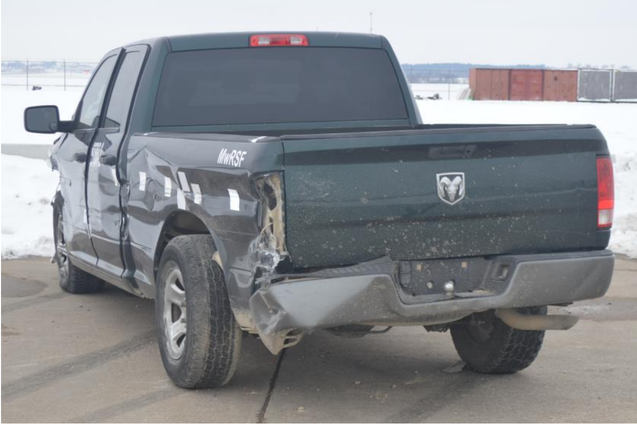
Figure 232. Vehicle Damage, Left-Corner Views, Test No. STBR-2
