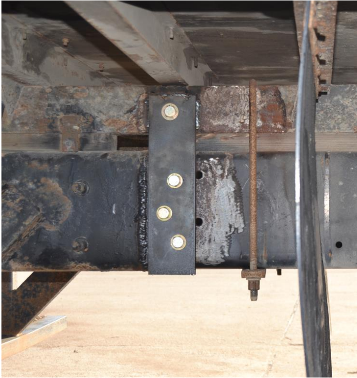
Left-Rear Shear Plate and U-Bolt
