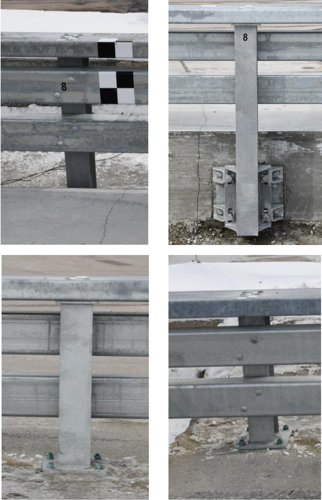
Figure 209. Test Installation Photographs, Side-Mounted and Top-Mounted Posts, Test No. STBR-2
