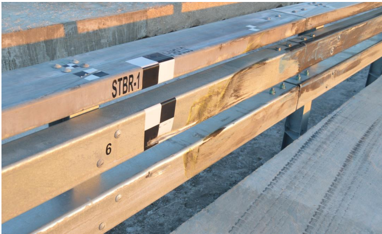
Figure 166. Damage to Rail Span Between Posts Nos. 6 and 7, Test No. STBR-1
