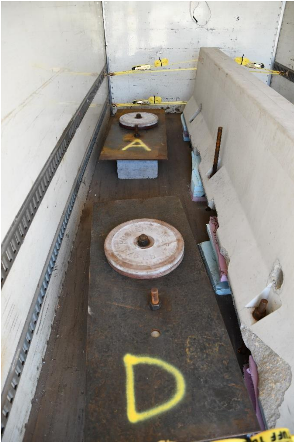
Figure 125. Nylon Straps and Ballast Installation, Test No. STBR-4
