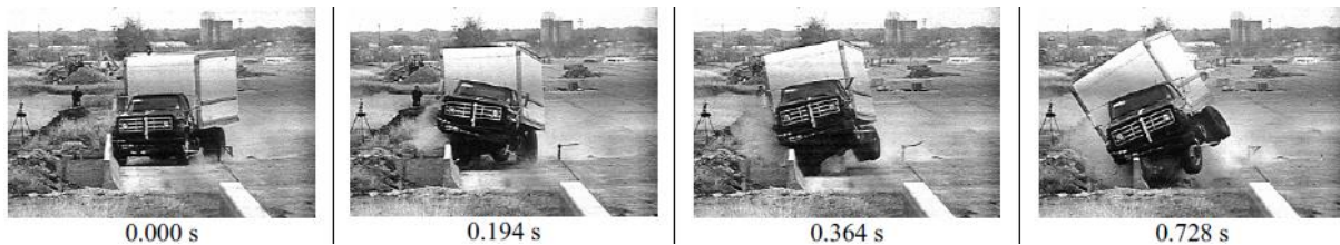
Figure 21. 32-in. Tall NJ Safety Shape Barrier under NCHRP 350 Impact Conditions [39]
