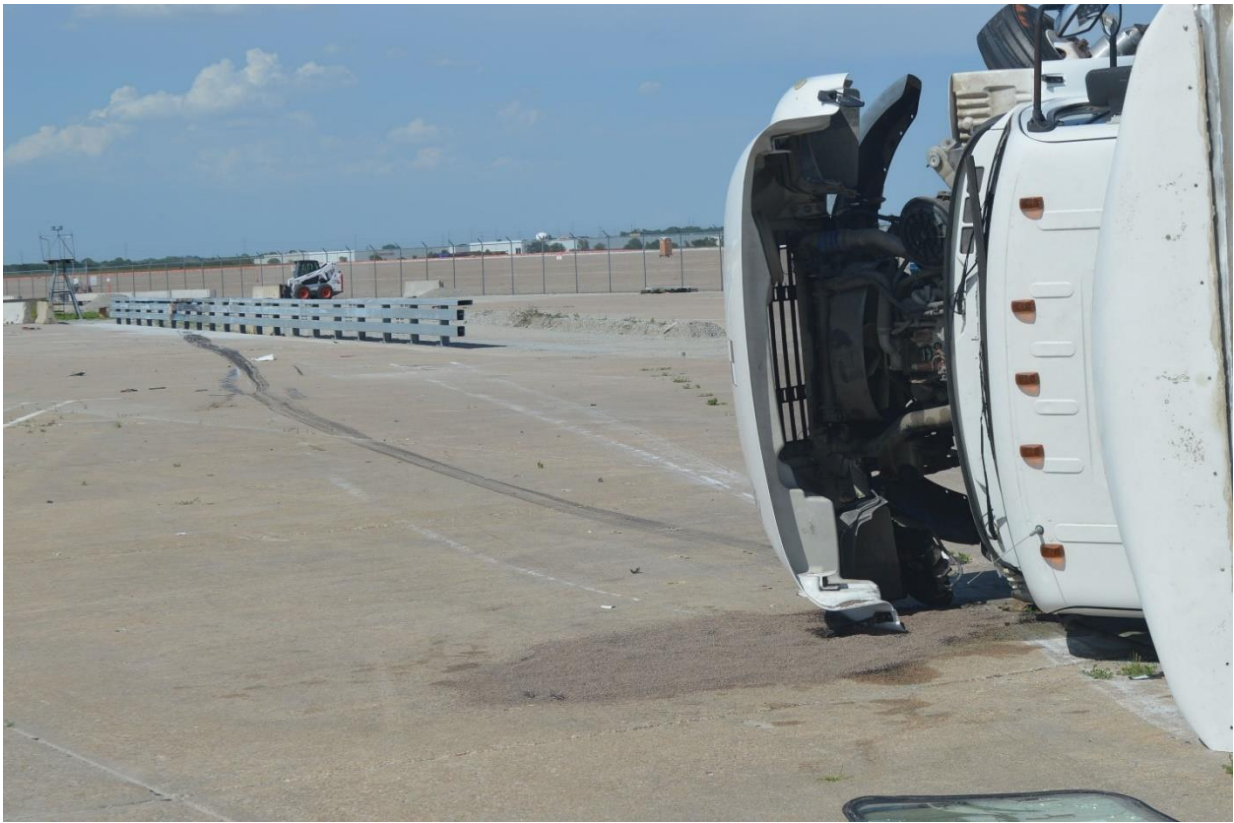
Figure 319. Vehicle Final Position and Trajectory Marks, Test No. STBR-4
