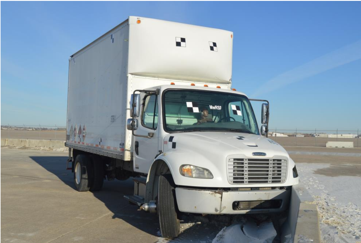
Figure 176. Vehicle Damage, Right Corner Views, Test No. STBR-1
