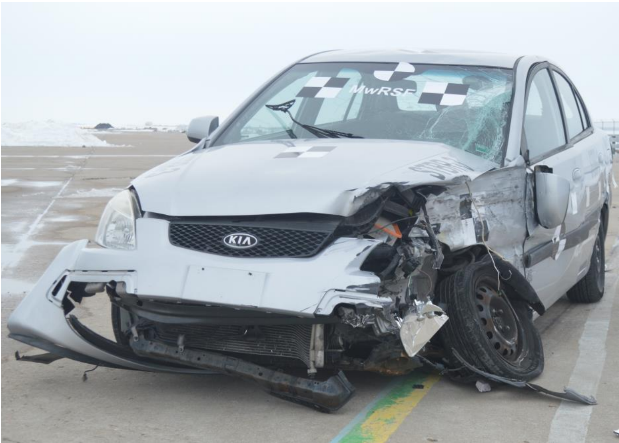
Figure 276. Vehicle Damage, Left Side, Test No. STBR-3
