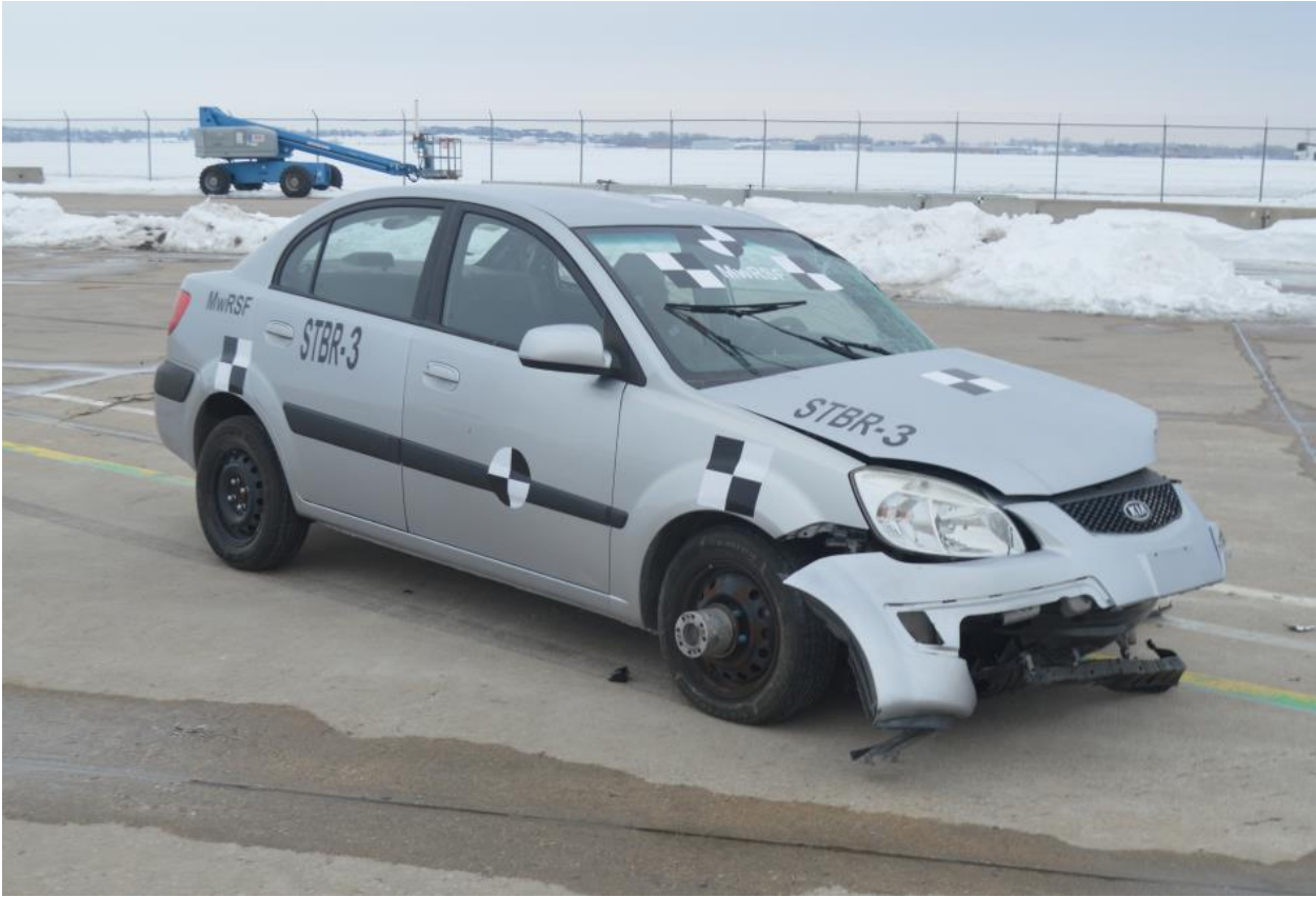
Figure 275. Vehicle Damage, Right Corner Views, Test No. STBR-3
