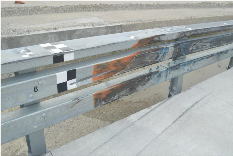
Figure 320. System Damage, Rail Span Between Posts Nos. 6 and 7, Test No. STBR-4
