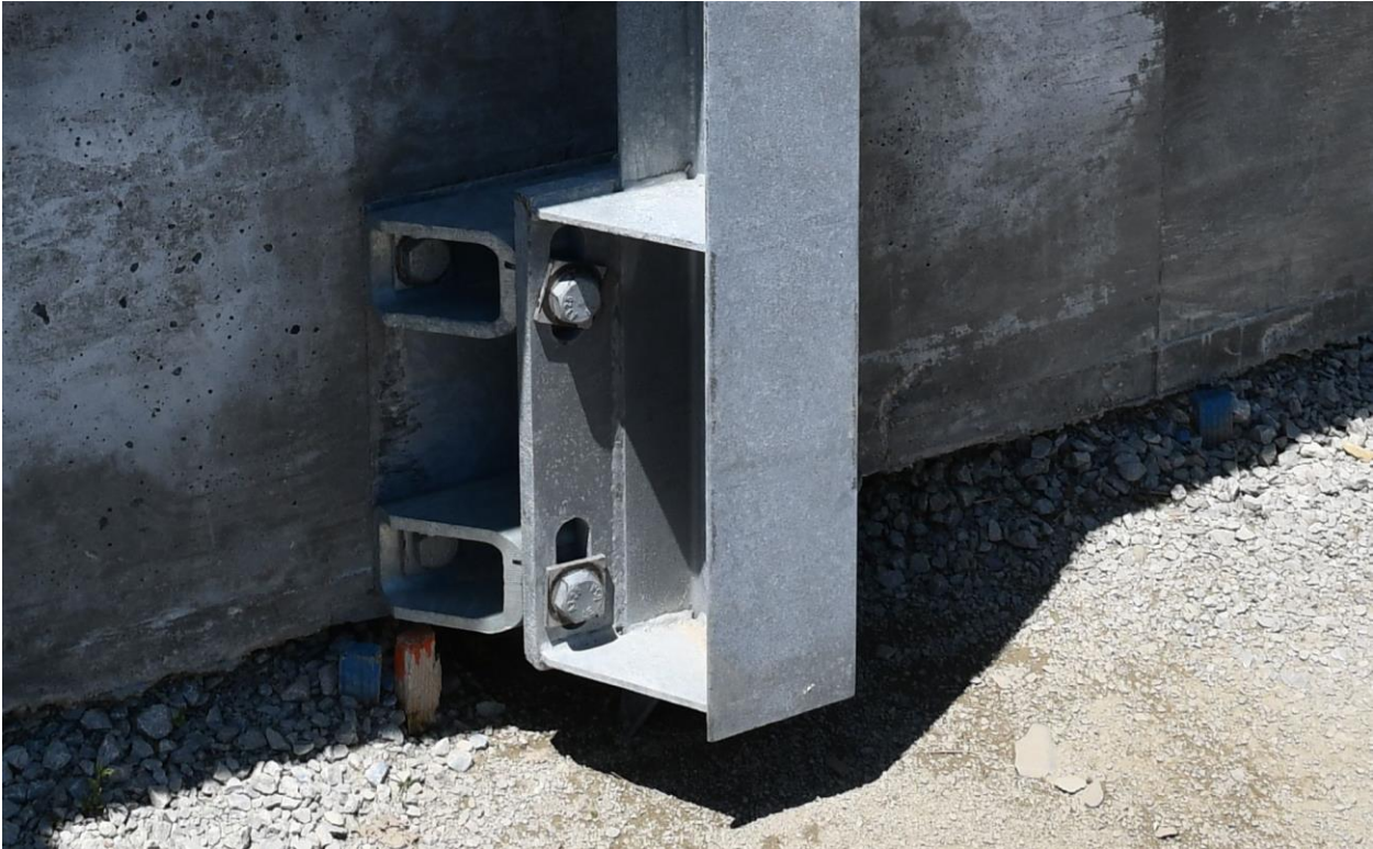
Figure 309. Side-Mounted Post-to-Deck Connections, Test No. STBR-4
