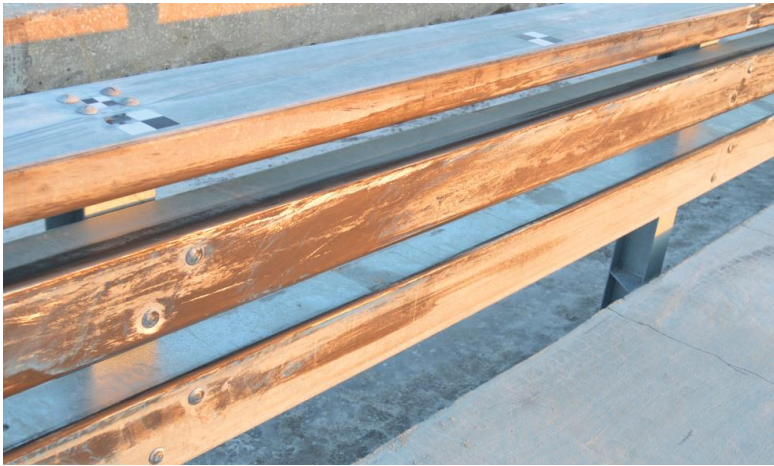
Figure 167. Damage to Rail Span Between Posts Nos. 7 and 8, Test No. STBR-1
