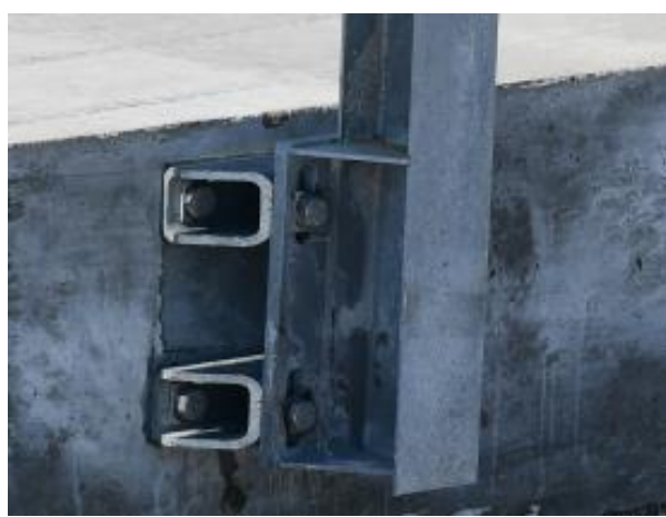
Figure 260. Test Installation Photograph, Side-Mounted Posts and Post-to-Deck Connections, Test No. STBR-3
