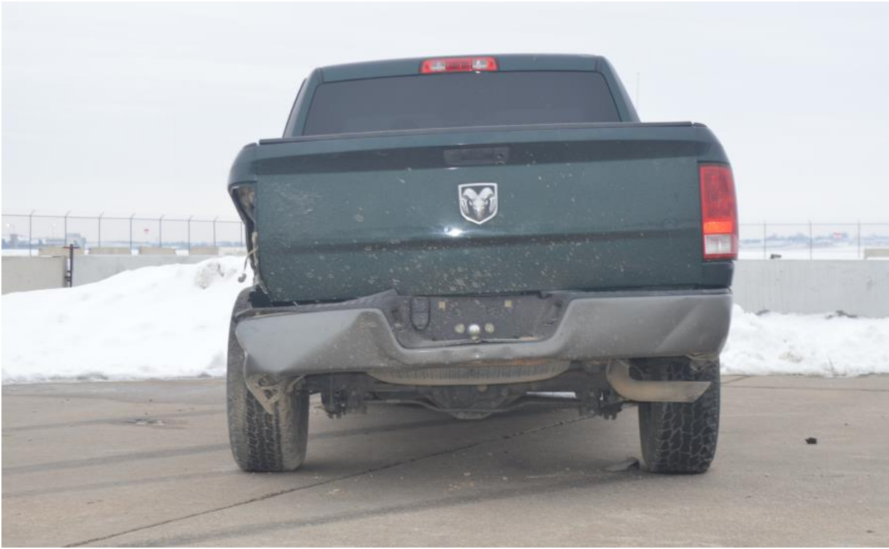
Figure 229. Vehicle Damage, Front and Rear Views, Test No. STBR-2
