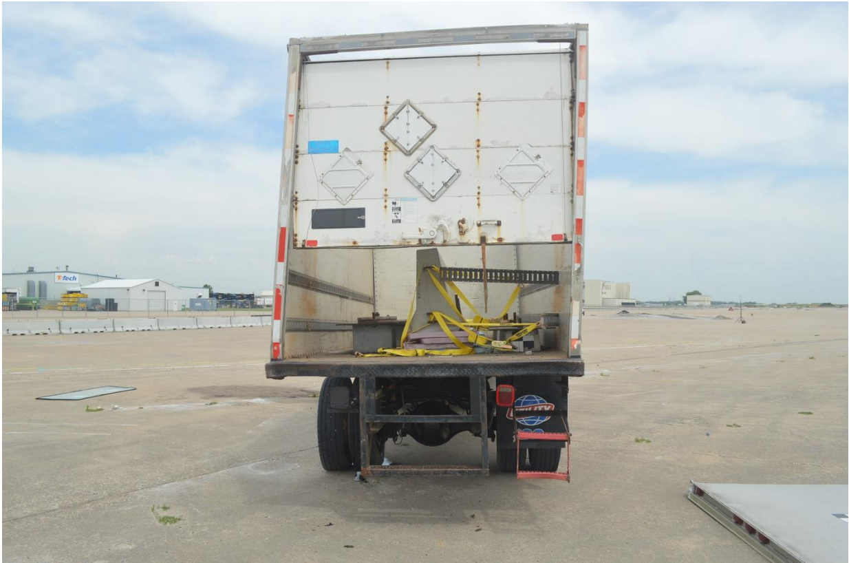
Figure 328. Vehicle Damage, Front and Rear Views, Test No. STBR-4
