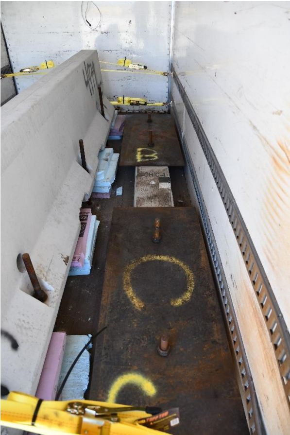
Figure 125. Nylon Straps and Ballast Installation, Test No. STBR-4
