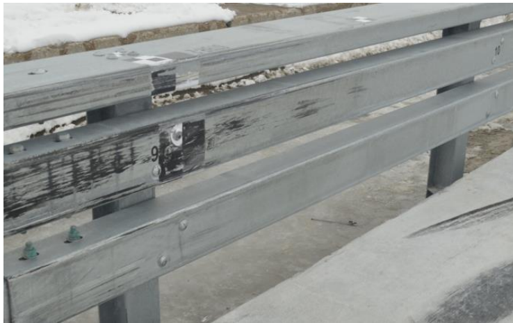
Figure 221. System Damage, Rail Span Between Posts Nos. 9 and 10, STBR-2
