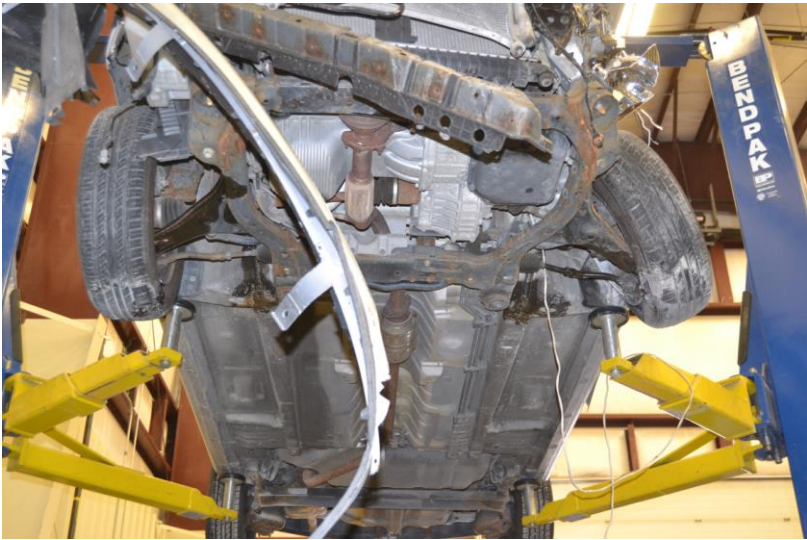
Figure 277. Vehicle Damage, Floor Pan and Undercarriage, Test No. STBR-3
