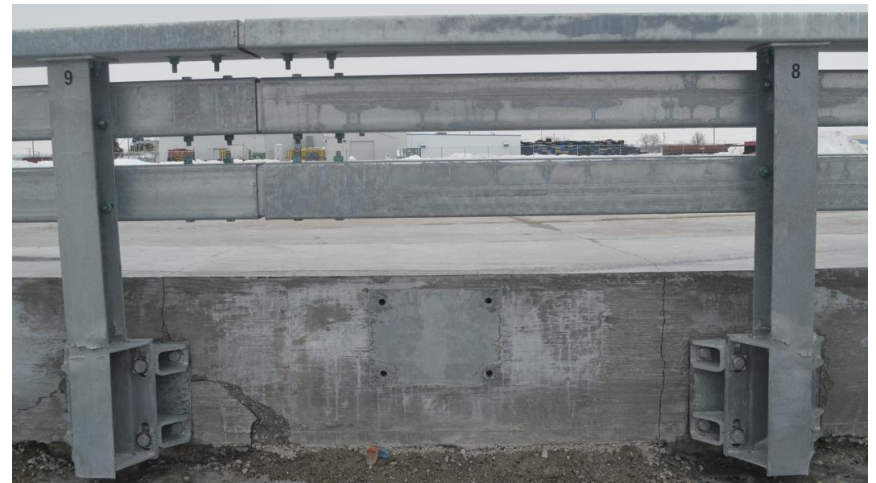
Figure 220. System Damage, Rail Span Between Posts Nos. 8 and 9, Test No. STBR-2
