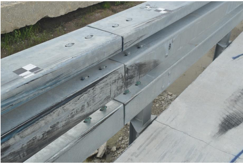
Figure 322. System Damage, Rail Span Between Posts Nos. 8 and 9, Test No. STBR-4
