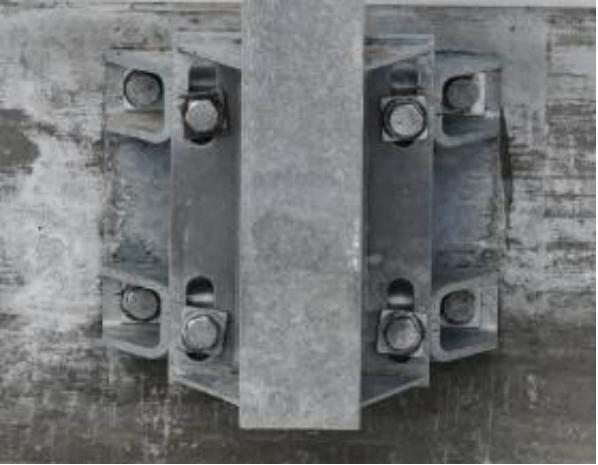
Figure 260. Test Installation Photograph, Side-Mounted Posts and Post-to-Deck Connections, Test No. STBR-3
