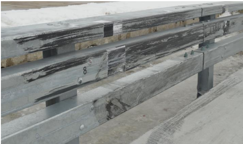
Figure 220. System Damage, Rail Span Between Posts Nos. 8 and 9, Test No. STBR-2
