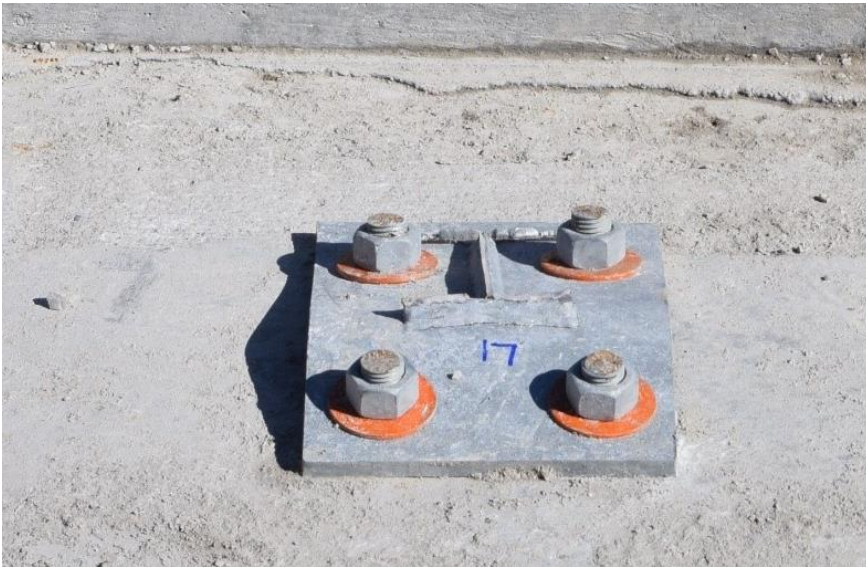
Figure 86. Damage to Base Plate Nos. 16 through 18 – After Soil Removal, Test No. CMGS-2
