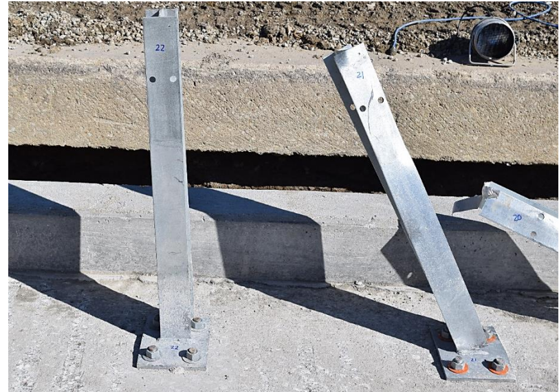
Figure 87. Damage to Post Nos. 17 through 22 Damage – After Soil Removal, Test No. CMGS-2
