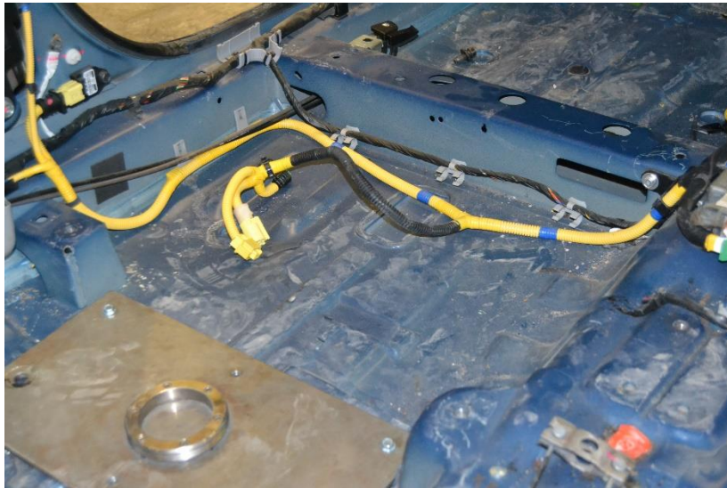
Figure 71. Occupant Compartment Damage, Test No. CMGS-1
