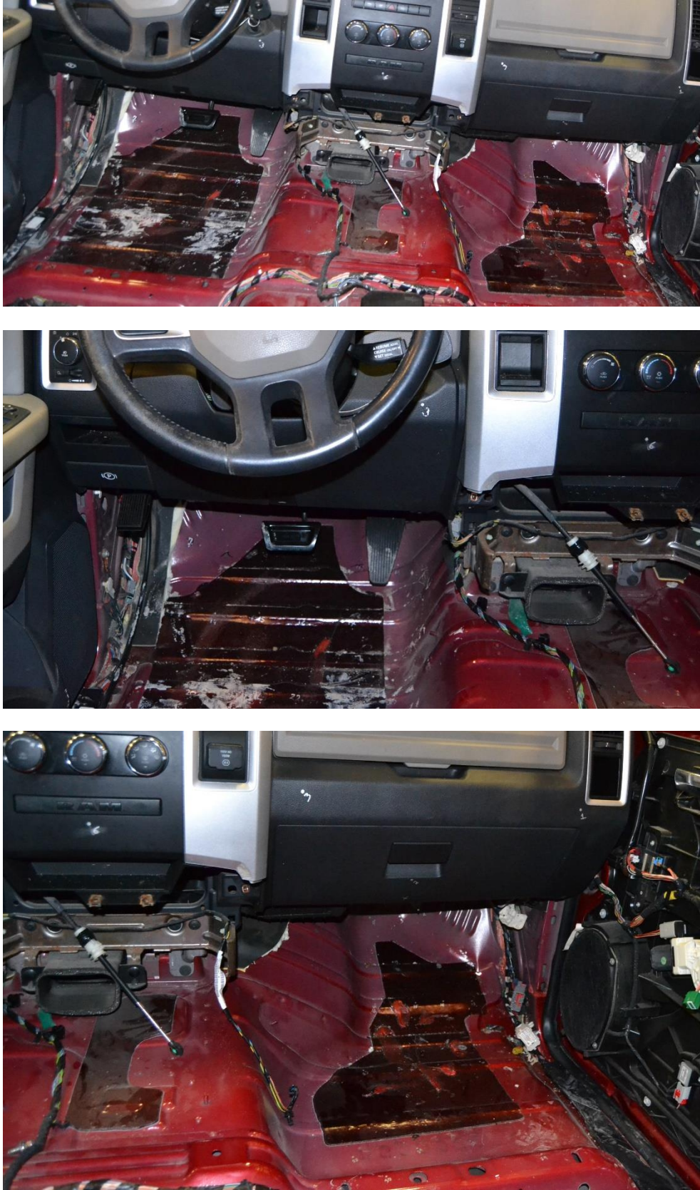
Figure 94. Vehicle Occupant Compartment Damage, Test No. CMGS-2
