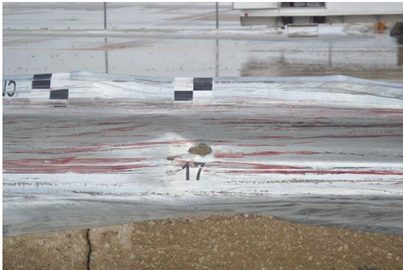
Figure 82. Guardrail Damage, Post Nos. 15 through 19, Test No. CMGS-2
