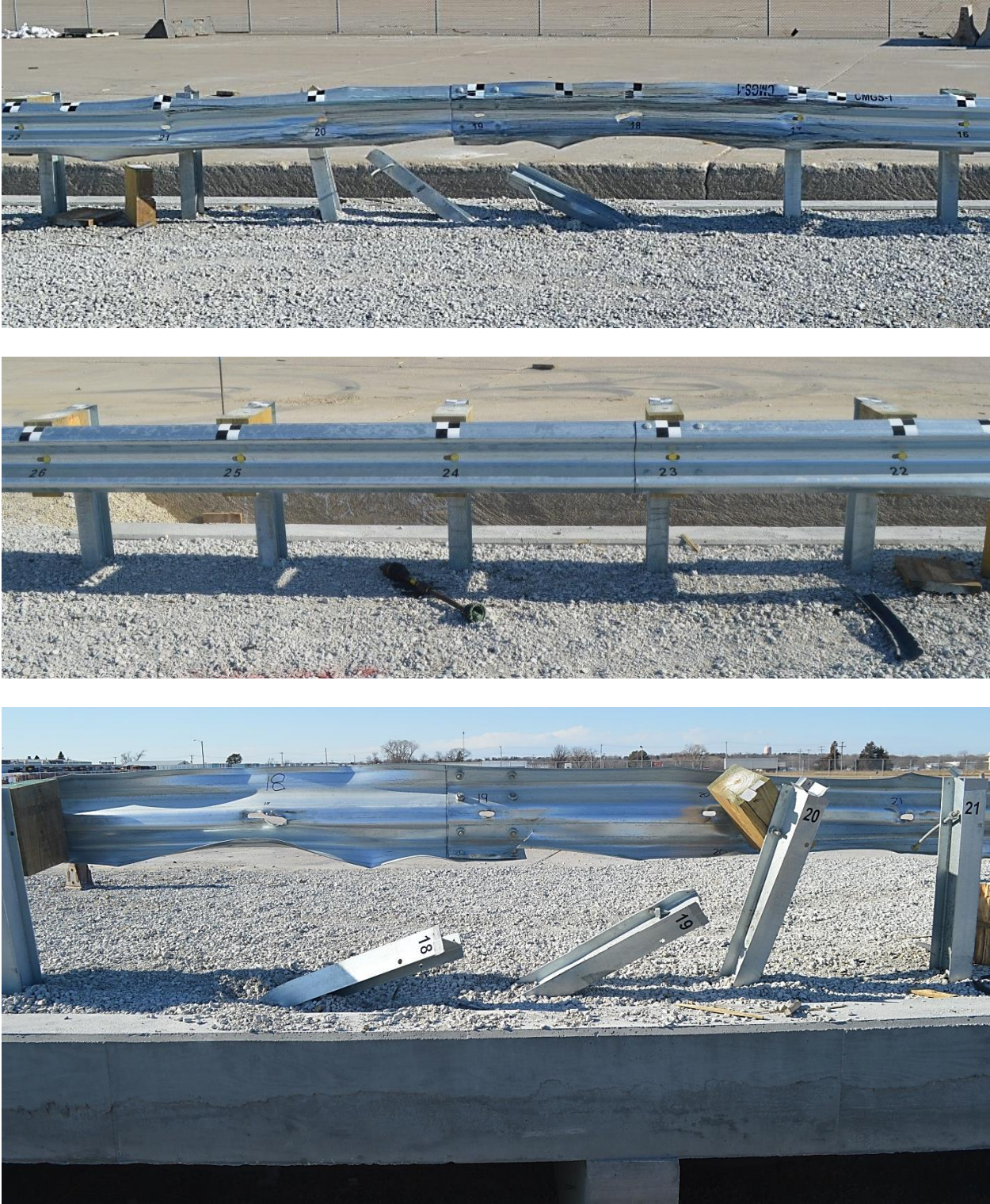
Figure 60. System Damage, Test No. CMGS-1
