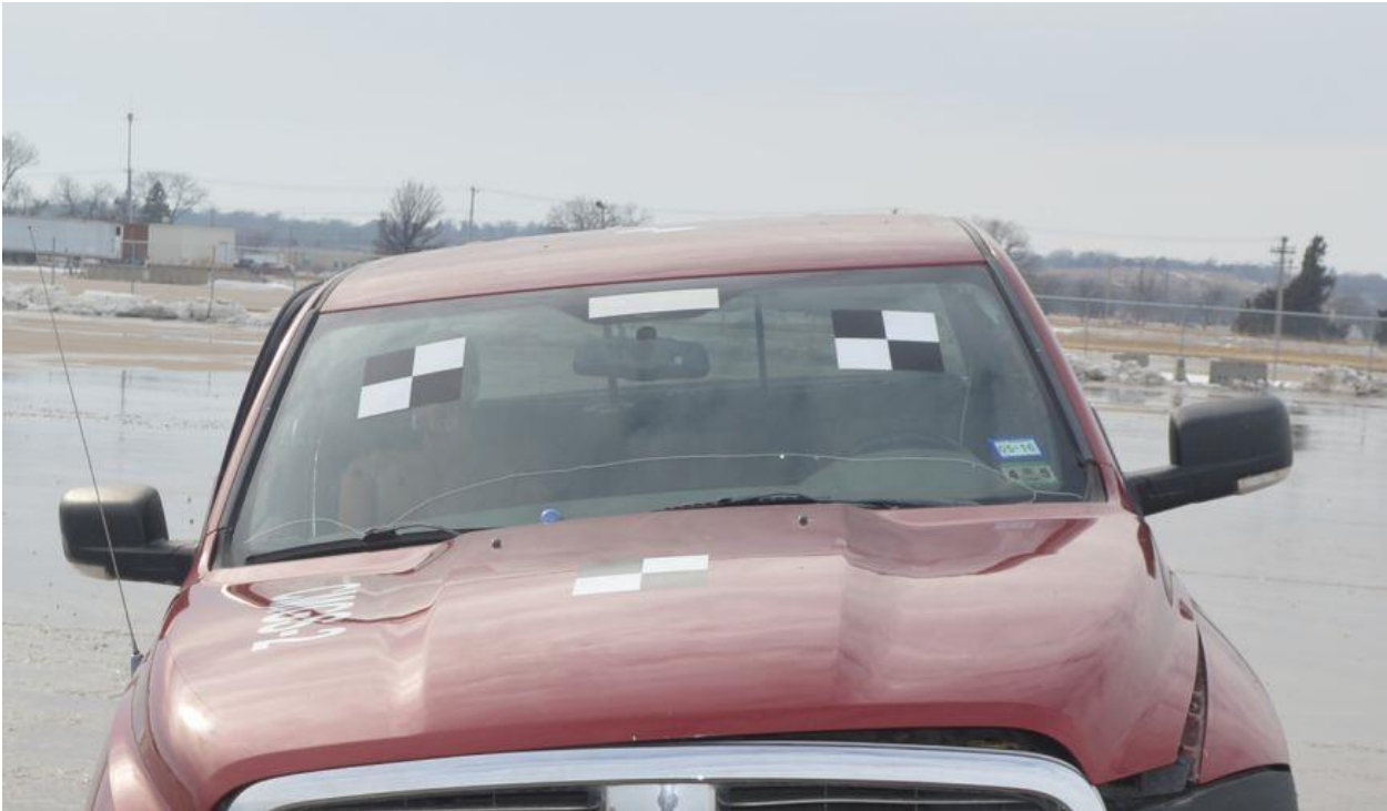
Figure 93. Vehicle Windshield Damage, Test No. CMGS-2
