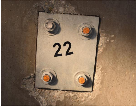
Figure 85. Damage to Base Plates of Post Nos. 17 through 22, Test No. CMGS-2
