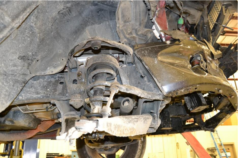
Figure 95. Vehicle Undercarriage Damage, Test No. CMGS-2
