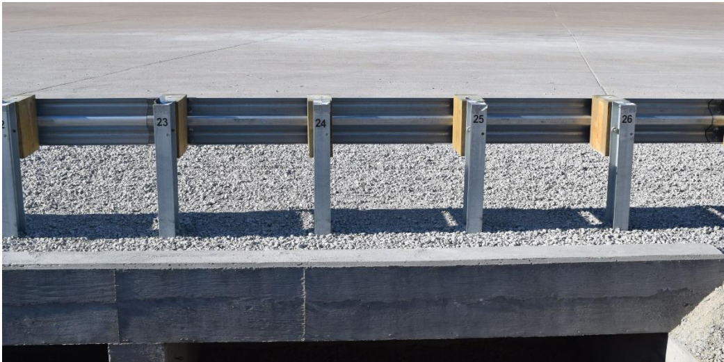
Figure 42. Posts Attached to Culvert, Test Nos. CMGS-1 and CMGS-2
