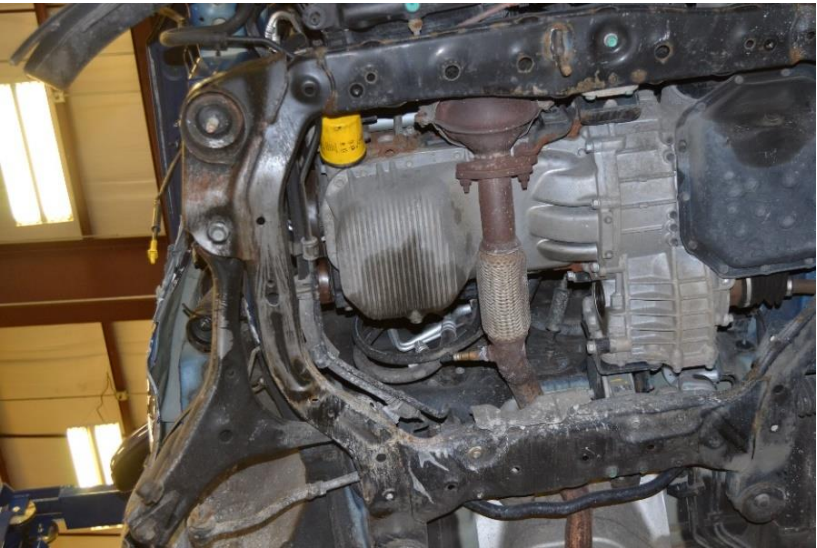
Figure 72. Vehicle Undercarriage Damage, Test No. CMGS-1
