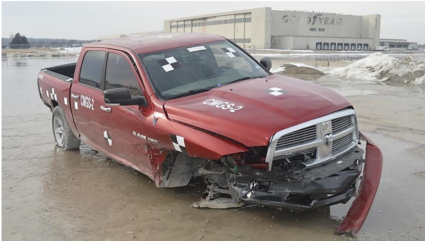
Figure 92. Additional Vehicle Damage, Test No. CMGS-2
