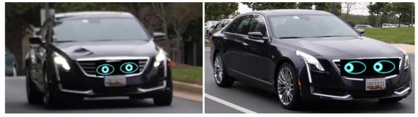
Figure 36. "I see you" eyes looking straight (left) and looking right (right)
