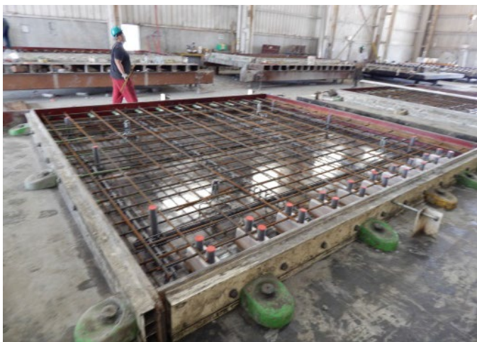
Figure 12. Typical reinforcement layout for a precast panel.
