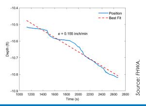
Soil layer's erosion rate (e) calculated from the slope of the best-fit line.
