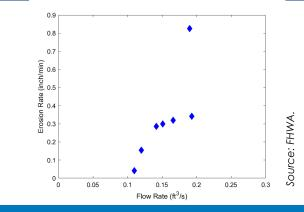
Erosion rate versus flow rate for the Lowndesboro ISTD demonstration. With more data points, a nonlinear fitted power curve could be used to extract the critical flow rate where erosion begins.
