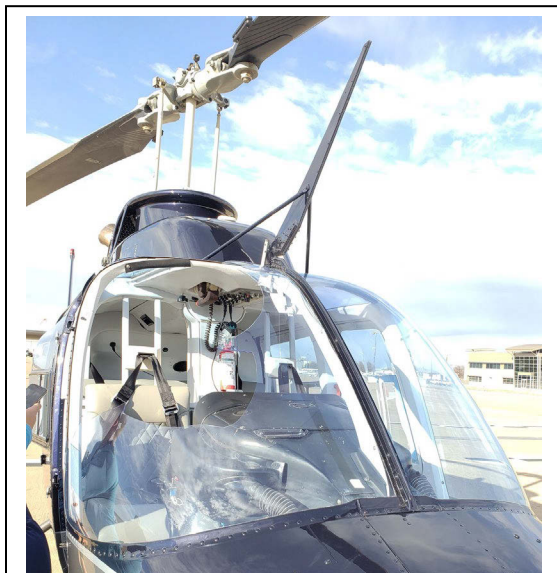
A Bell 206 helicopter en route at 105 knots and 1,200 feet above ground level struck a soaring red-tailed hawk in Texas, January 2019. The hawk penetrated windshield. The pilot, with minor injuries, made an emergency landing at nearby airport with dead hawk in his lap. Photo, aircraft owner.
