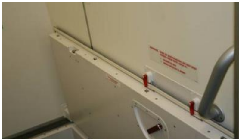
Figure 83. Airtight Hatch Door to A380 Lower-Deck Crew Rest Area (Photograph courtesy of FAA)
