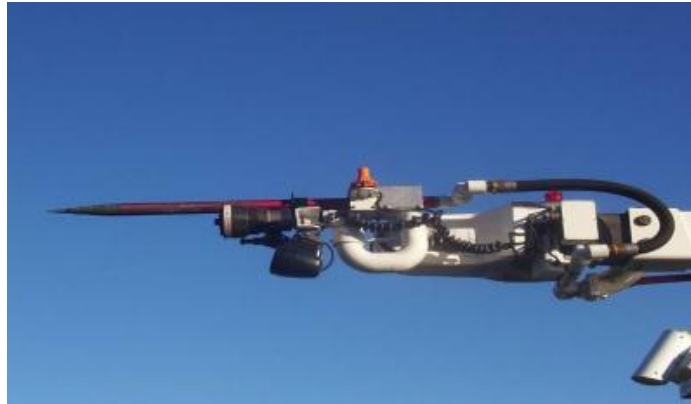
Figure 122. The HRET Using Boom Hydraulics for Penetration (Photograph courtesy of FAA)
