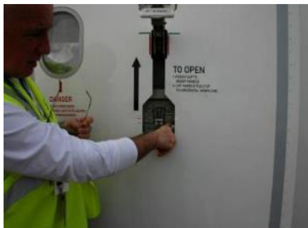
Figure 35. The A380 ML1 Door, Exterior Operation Demonstration—Step 7 (Photograph courtesy of FAA)
