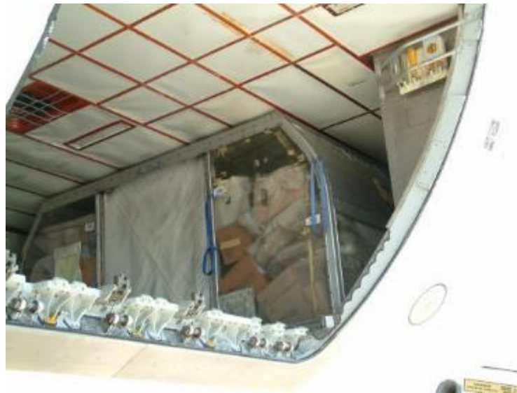
Figure 145. A ULD in Position in Lower Cargo Compartment (Photograph courtesy of FAA)
