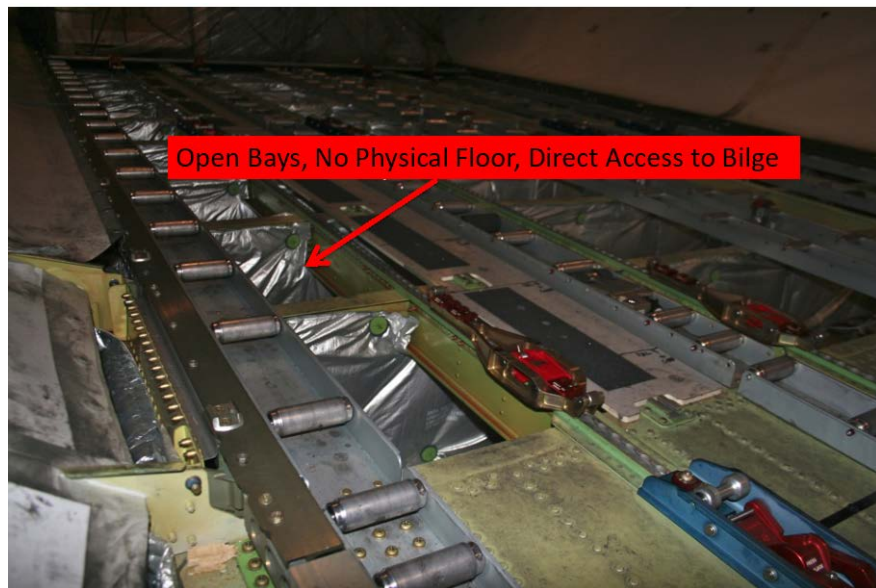
Figure 152. Open Bays in Cargo Floor—B-747-8I (Photograph courtesy of FAA)
