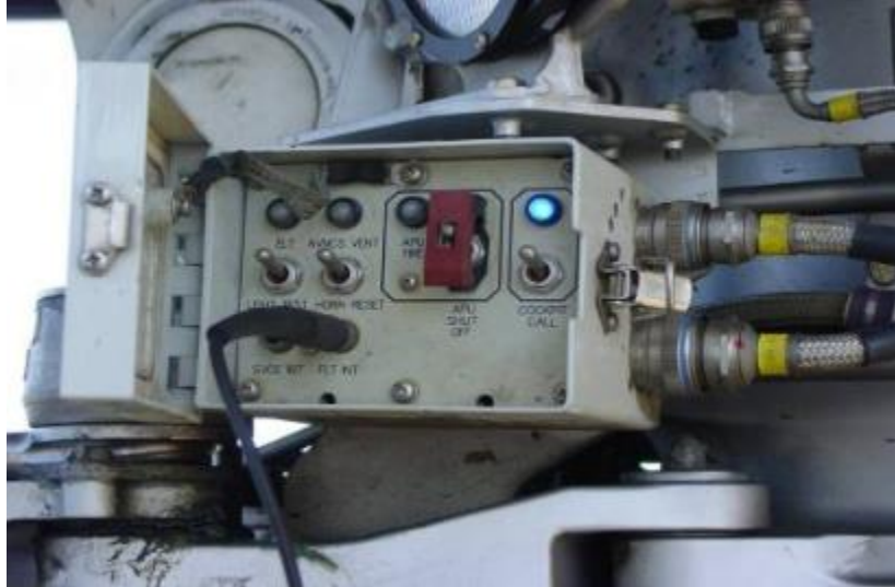
Figure 170. Nose Gear APU Panel (Photograph courtesy of FAA)
