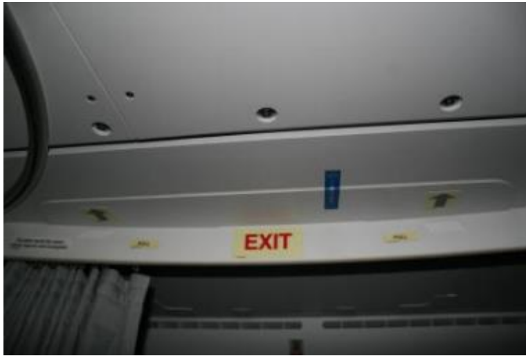
Figure 86. Secondary Exit From Lower-Deck Crew Rest Facility, Lufthansa A380 (Photograph courtesy of FAA)
