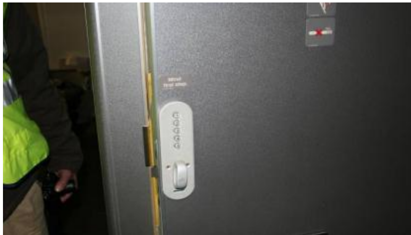
Figure 81. Access Door From Main Deck to Lower-Deck Crew Rest Facility (FAA Photograph)
