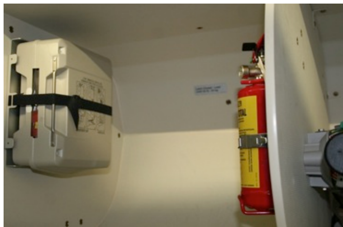
Figure 63. Fire Extinguisher Mounted in Overhead Bin on B-747-8I (Photograph courtesy of FAA)
