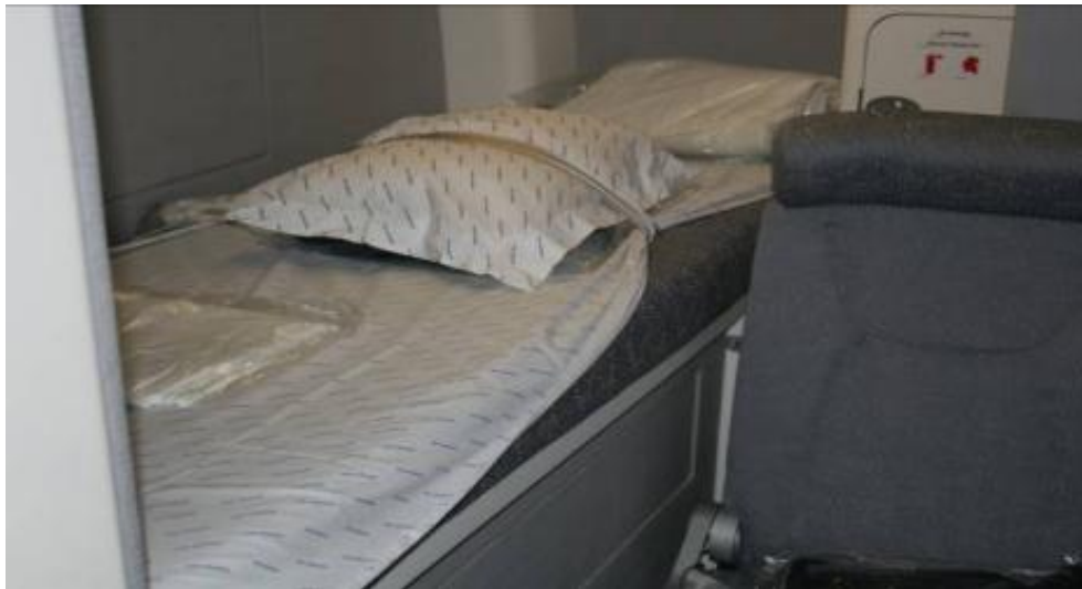
Figure 89. Main-Deck Flight Crew Rest Facility Located Aft of Cockpit (Photograph courtesy of FAA)
