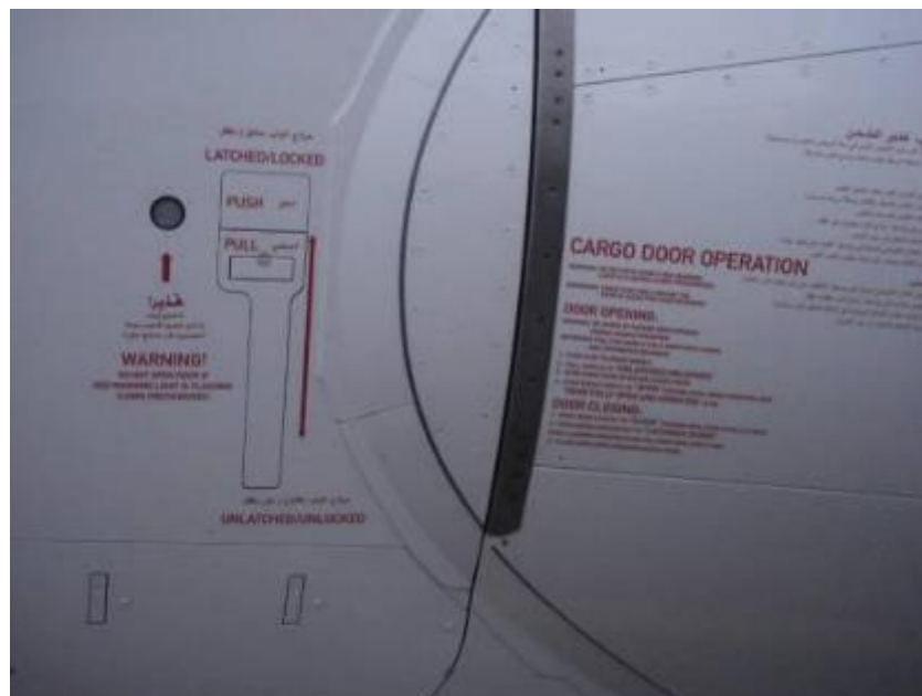
Figure 150. Aft Cargo Door Operation (Photograph courtesy of FAA)
