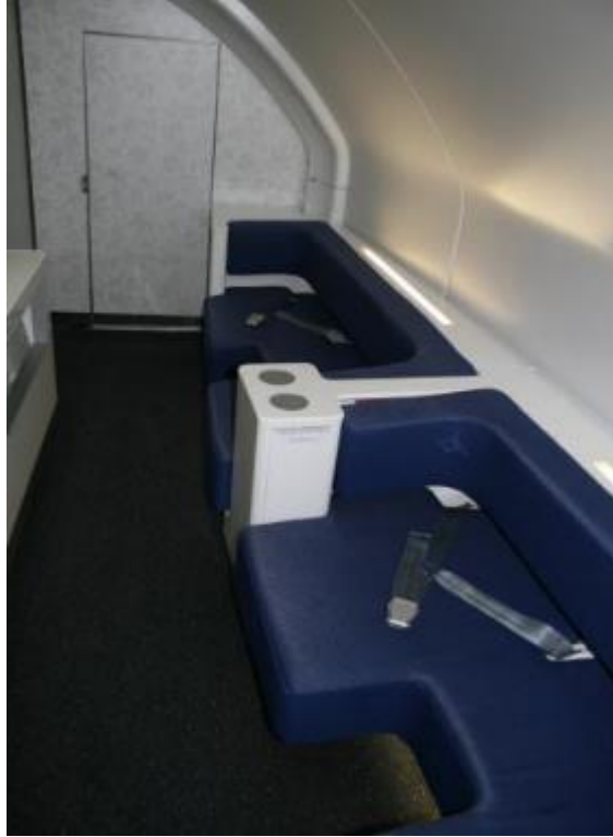
Figure 74. The A380 Access to Upper-Deck Avionics From Lounge/Seating Area (Photograph courtesy of FAA)
