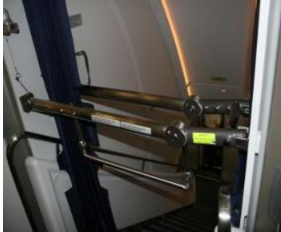
Figure 107. Gate in Operational Position, A380 Top of Main Passenger Stairs (Photograph courtesy of FAA)
