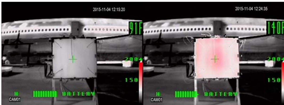
Figure 128. Hot Spot Identification for Carbon Fiber (Photograph courtesy of FAA (2017))
