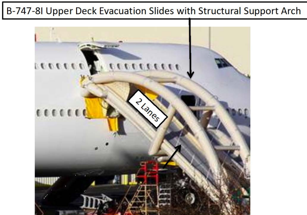
Figure 7. Structural Support Arch on B-747-8I Upper-Deck Slides (Photograph courtesy of Paine Field Blog 1-5-2012)
