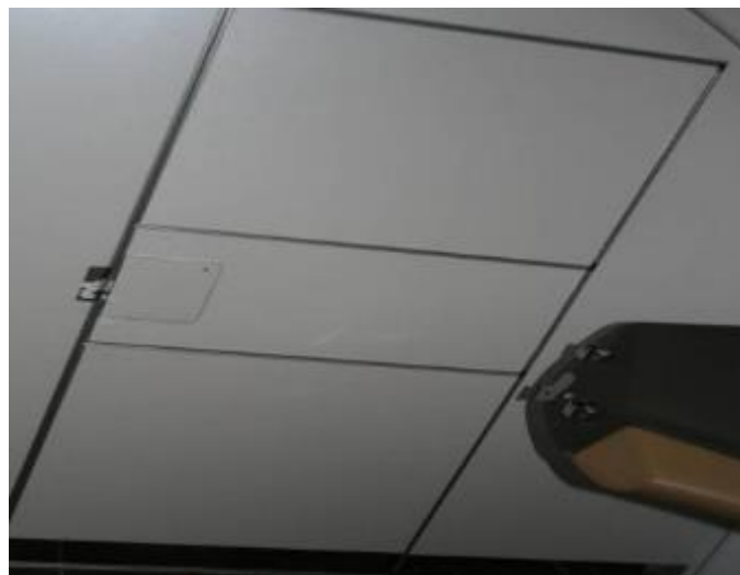
Figure 73. The A380 Upper Avionics Bay With Leaning Rail Raised, Exposing the Locked Door (Photograph courtesy of FAA)
