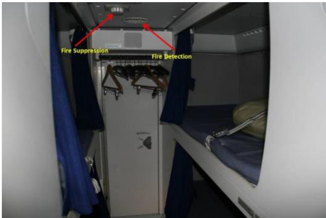
Figure 88. Lower-Deck Crew Rest Area Fire Detection and Suppression (Photograph courtesy of FAA)
