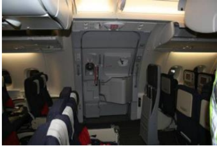
Figure 111. Obstructions to Direct Attack Through Entry Doors (Photograph courtesy of FAA)
