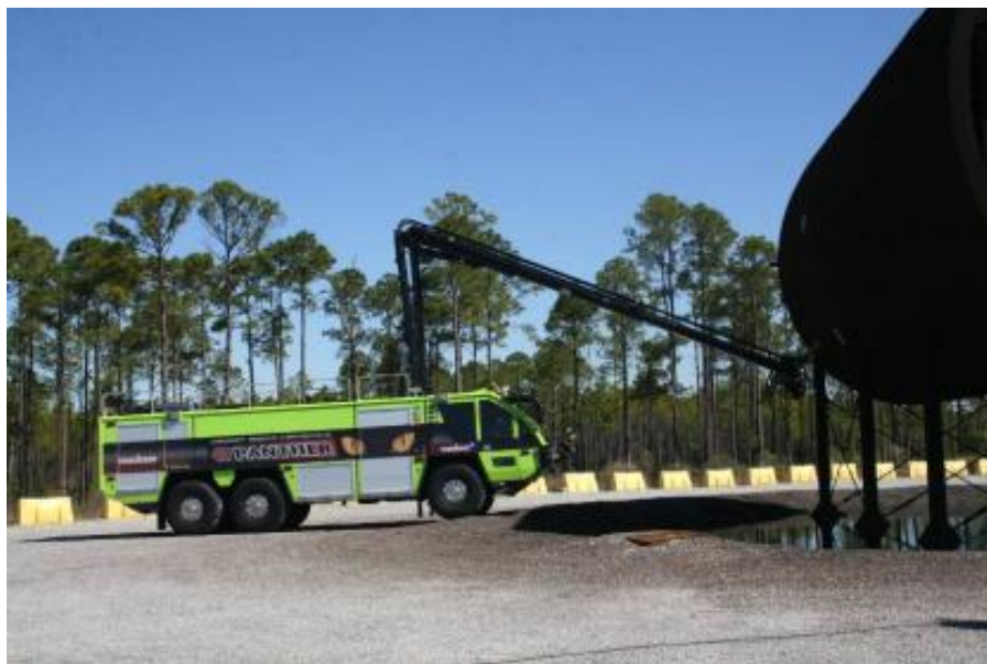
Figure 138. Positioning With Increased Standoff Distance (Photograph courtesy of FAA)
