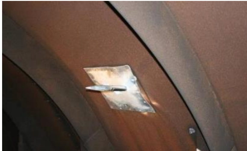
Figure 137. Proper Piercing Angle on Steeper Slope of Fuselage (Photograph courtesy of FAA)
