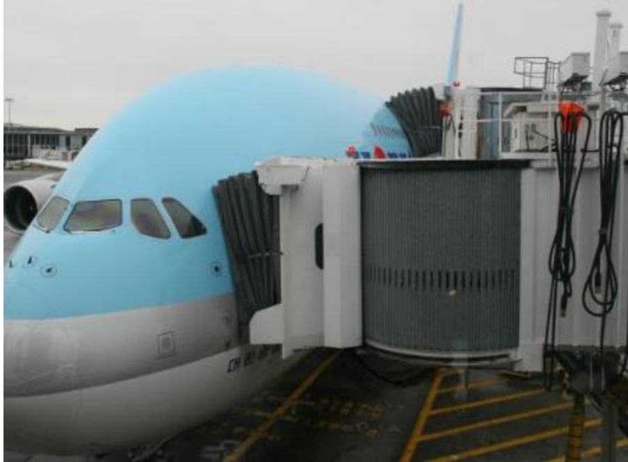
Figure 48. Korean A380 With Two Jet Bridges Extended at JFK (Photograph courtesy of FAA)
