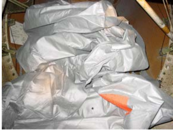
Figure 22. Evacuation Slide Deployment MD-81—Tail Cone (Image courtesy of NTSB)
