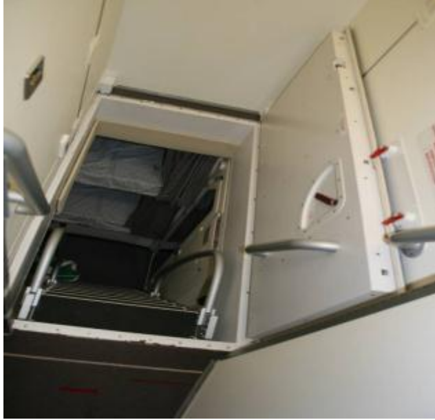
Figure 82. Access Ladder to A380 Lower-Deck Crew Rest Area (Photograph courtesy of FAA)
