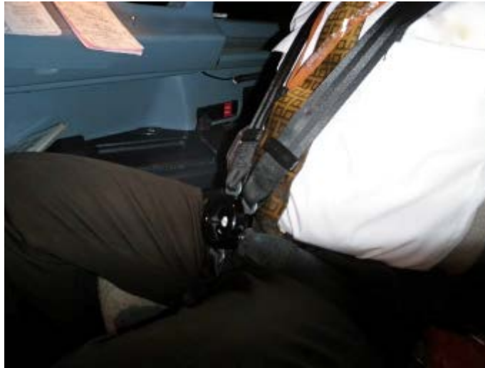
Figure 58. Five-Point Restraint (Photograph courtesy of IPA)
