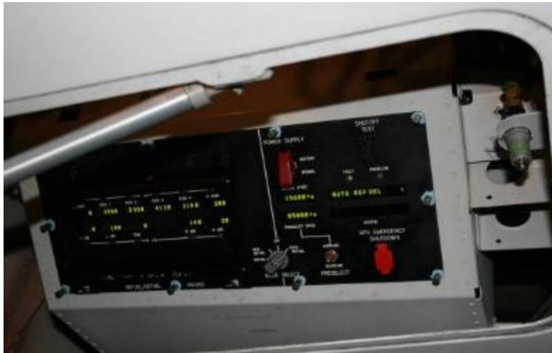
Figure 169. The APU Emergency Shutdown Controls in the Refuel/Defuel Panel (Photograph courtesy of FAA)
