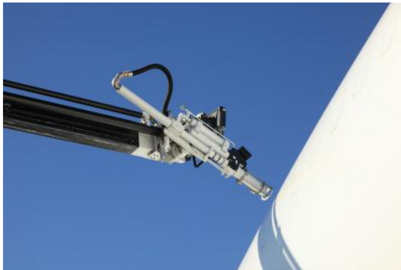
Figure 123. The HRET Using Hydraulic Accumulators for Penetration (Photograph courtesy of FAA)
