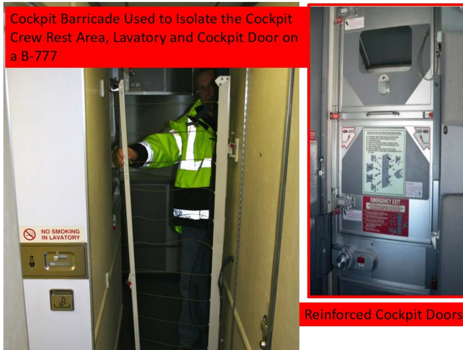
Figure 53. Reinforced Cockpit Barricade and Doors on a B-777
