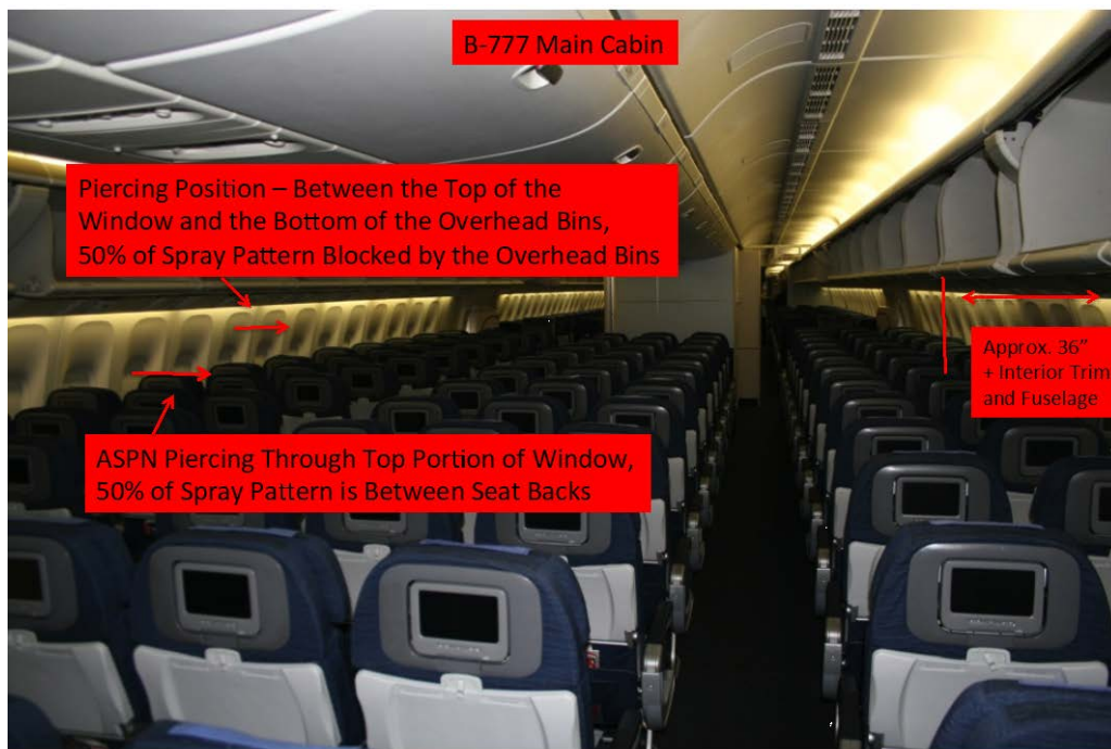
Figure 121. Limitations of the ASPN in a B-777 Main Cabin (Photograph courtesy of FAA)
