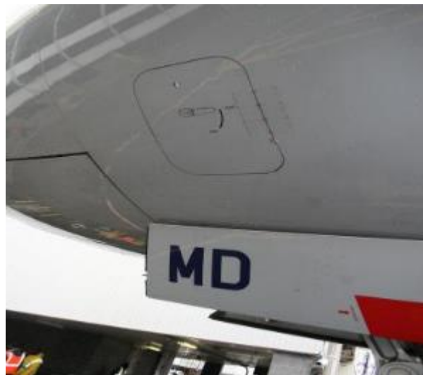
Figure 71. Access Hatch From Forward Fuselage Left Side to Main Avionics Bay (Photograph courtesy of FAA)
