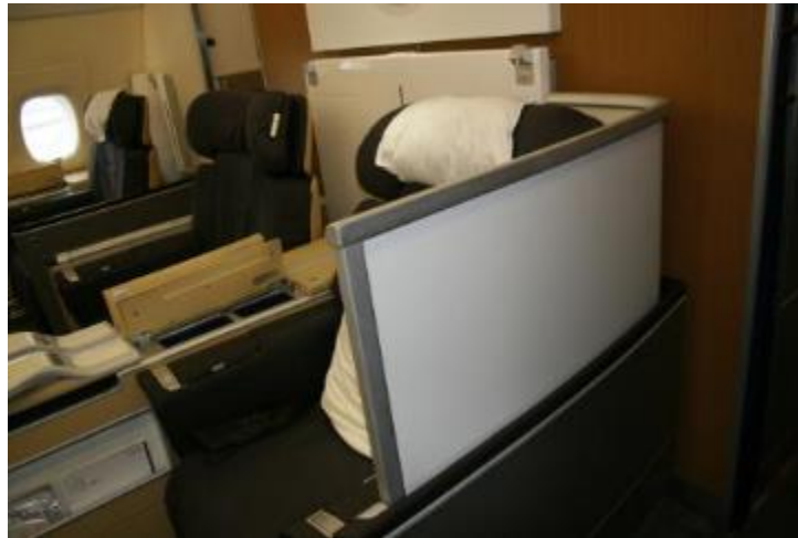
Figure 176. Raised Partition Around First-Class Seat on Lufthansa A380
