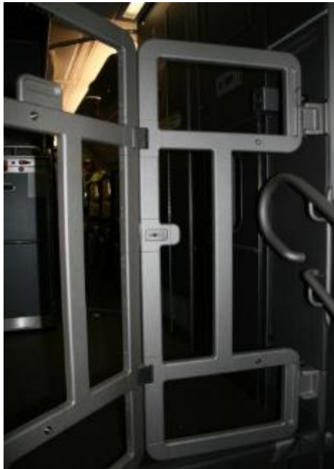
Figure 104. Gate at Top of Rear Service Stairs, A380 Upper Deck (Photograph courtesy of FAA)
