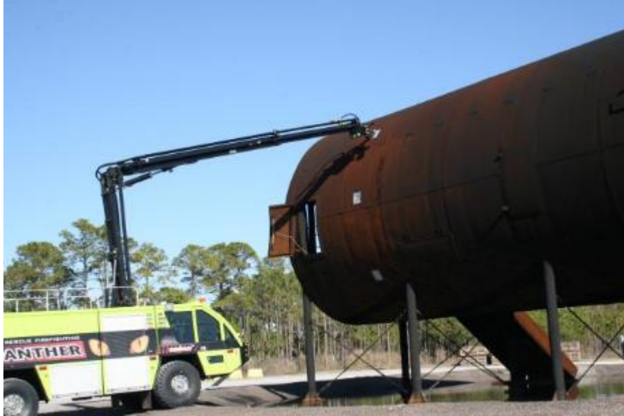
Figure 135. Standoff Position and Approach for Upper-Deck Piercing (Photograph courtesy of FAA)
