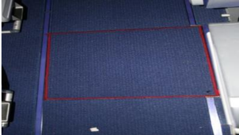
Figure 87. Emergency Escape Hatch From Lower-Deck Crew Rest Facility, Lufthansa A380 (Photograph courtesy of FAA)
