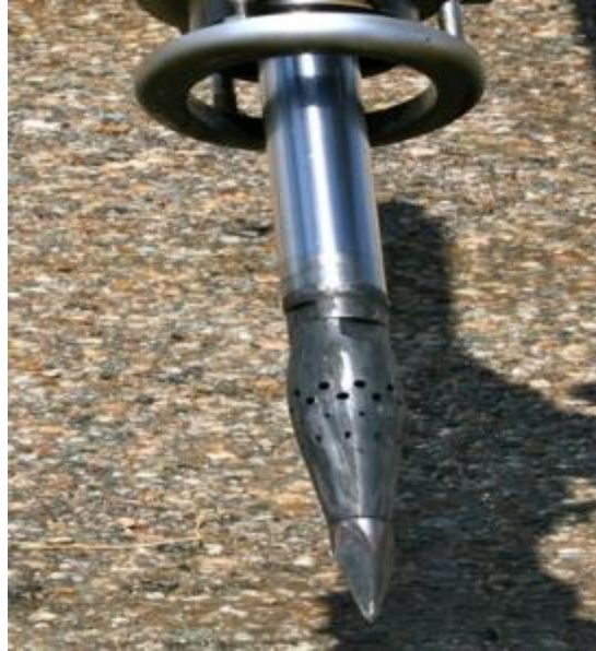
Figure 120. Agent Discharge Holes on Rosenbauer Stinger ASPN (Photograph courtesy of FAA)
