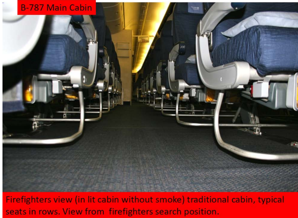
Figure 47. Typical Firefighter View in Traditional B-787 Main Cabin Without Smoke (Photograph courtesy of FAA)
