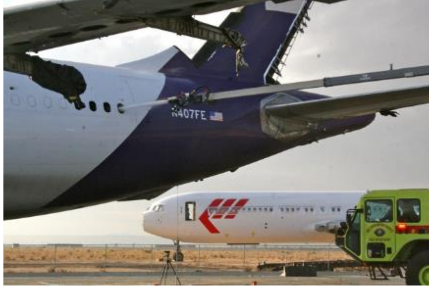
Figure 134. The HRET Turret Discharge (1000 gpm) Through Window Removed by ASPN (Photograph courtesy of FAA)
