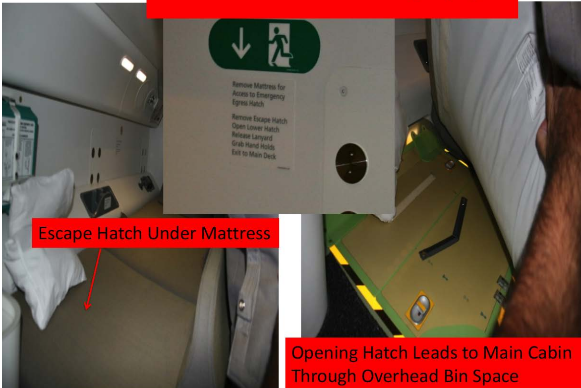
Figure 97. The B-787 Overhead Crew Rest Emergency Egress
