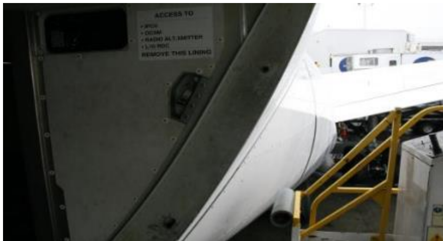
Figure 142. Flare of Fairing Between Cargo Compartment and Wing (Photograph courtesy of FAA)
