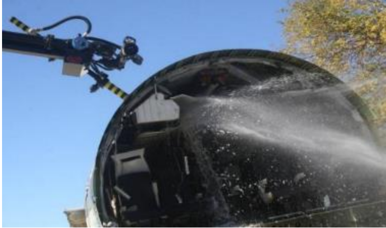
Figure 131. Testing to Understand the Effect of Piercing the Overhead Bin (Photograph courtesy of FAA (2010))
