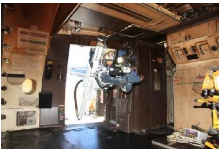
Figure 125. Testing the FAA HRET (Photograph courtesy of FAA)
