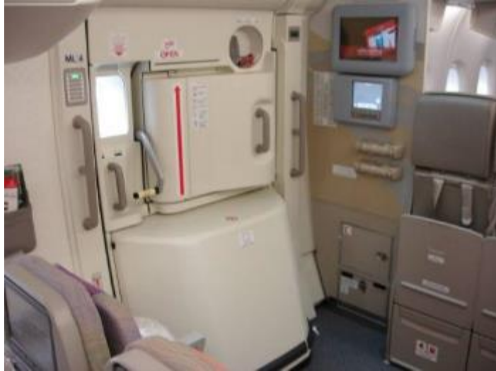
Figure 32. The A380 ML4 Door, Interior View: Type A Passenger Door With Slide Container (Photograph courtesy of FAA)
