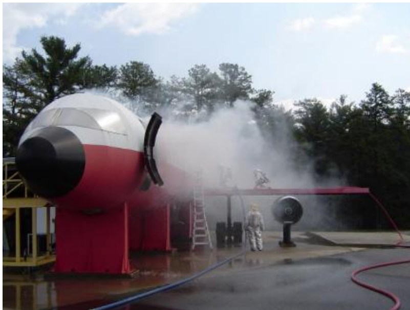
Figure 112. Fire Attack Resulting in Horizontal Ventilation During ARFF Training (Photograph courtesy of Jeremy Souza PVD ARFF)
