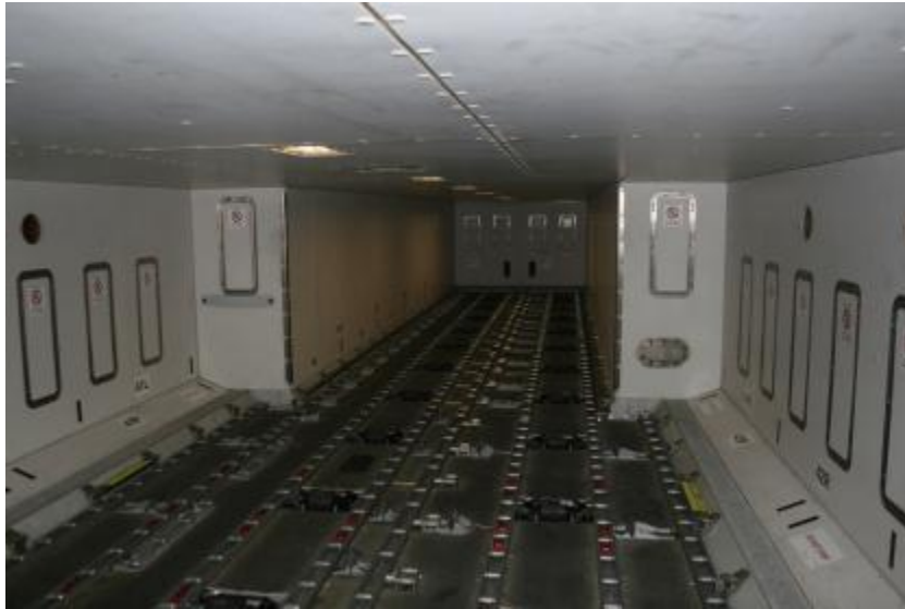
Figure 139. Forward Portion of Aft Cargo Compartment, Known as the Tunnel (Photograph courtesy of FAA)
