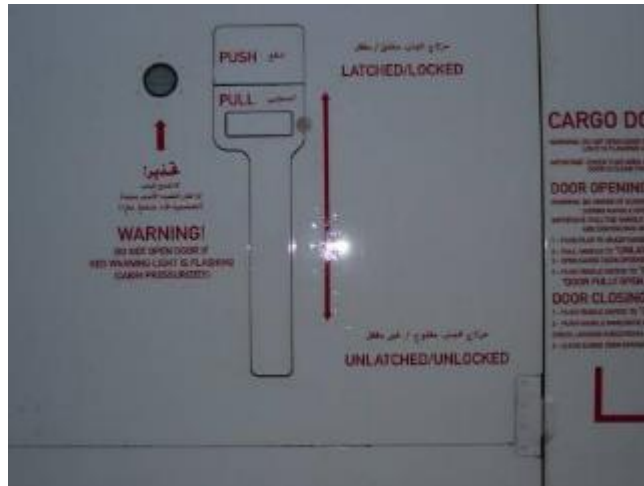
Figure 149. Forward Cargo Door Operation (Photograph courtesy of FAA)
