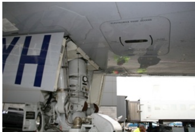
Figure 68. Access Hatch to E&E Compartment on B-747-8 (Photograph courtesy of FAA)
