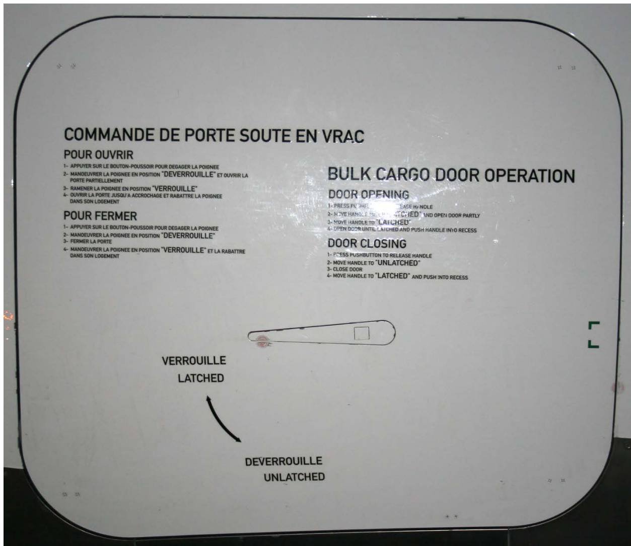
Figure 148. Bulk Cargo Door Operation (Photograph courtesy of FAA)
