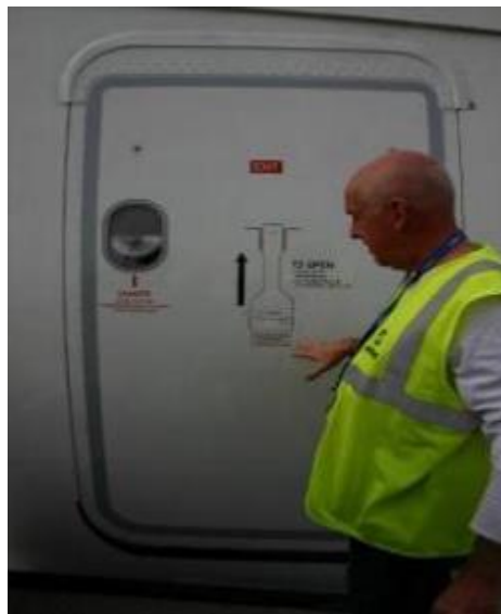
Figure 33. The A380 ML1 Door, Exterior Operation View (Photograph courtesy of FAA)
