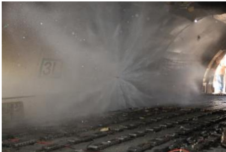
Figure 124. Discharge Pattern of ASPN on HRET (Photograph courtesy of FAA)
