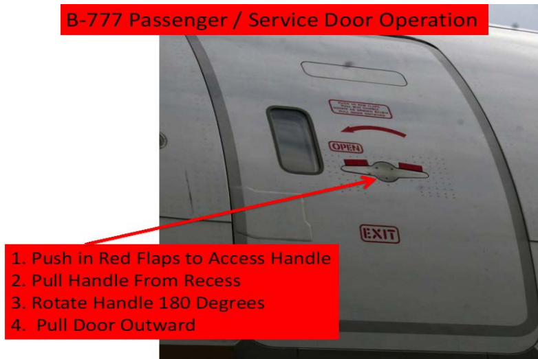
Figure 36. The B-777 Passenger/Service Door Operation (Photograph courtesy of FAA)
