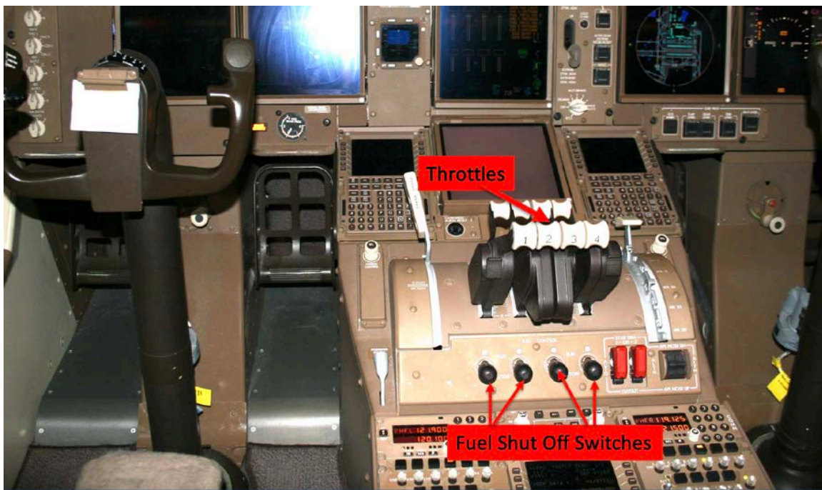
Figure 50. The B-747-81 Throttles and Fuel Shutoff Switches (Photograph courtesy of FAA)
