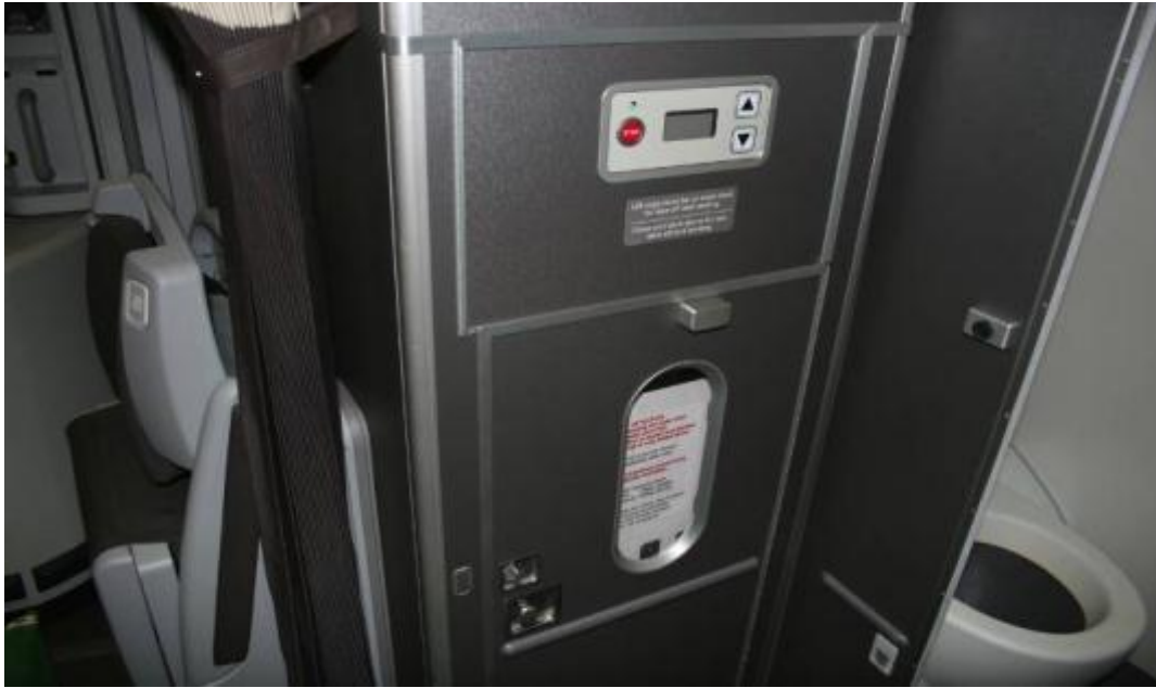
Figure 26. Service Elevator on Air France A380 (Photograph courtesy of FAA)
