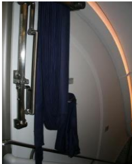
Figure 106. Gate and Curtain Stowed Position, A380 Main Passenger Stairs (Photograph courtesy of FAA)
