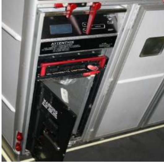
Figure 99. The A380 Galley Trash Compactor (Photograph courtesy of FAA)
