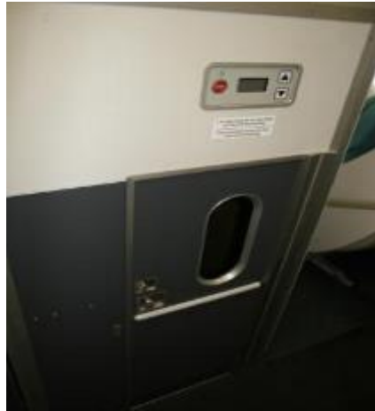
Figure 102. The A380 Galley Service Elevator (Photograph courtesy of FAA)
