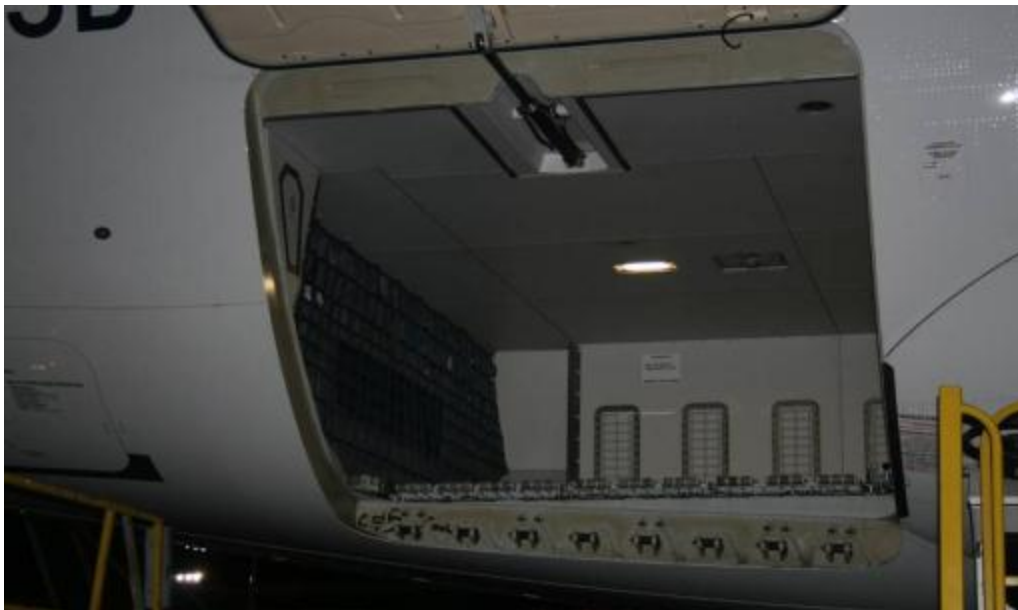
Figure 144. Aft Cargo Compartment With Cargo Net Separating the Bulk Cargo Compartment (Photograph courtesy of FAA)
