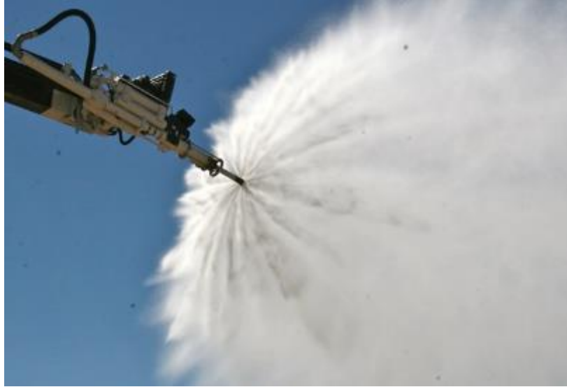
Figure 133. The ASPN Spray Pattern on Rosenbauer Stinger (ASPN) (Photograph courtesy of FAA)
