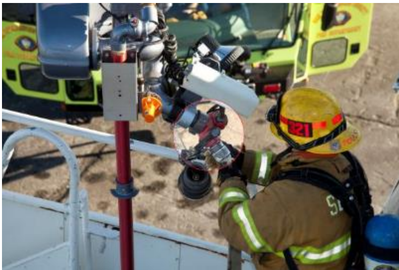
Figure 110. Firefighter Using the HRET Boom as a Waterway (Photograph courtesy of FAA)
