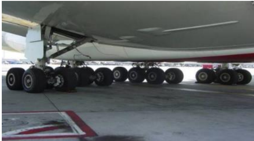
Figure 157. The A380 WLG and BLG—View From Front (Photograph courtesy of FAA—Taken from right side of aircraft)
