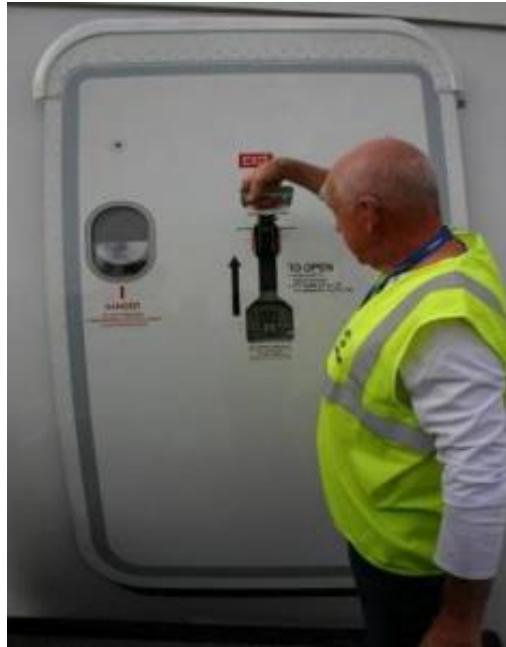
Figure 34. The A380 ML1 Door, Exterior Operation Demonstration—Step 6 (Photograph courtesy of FAA)
