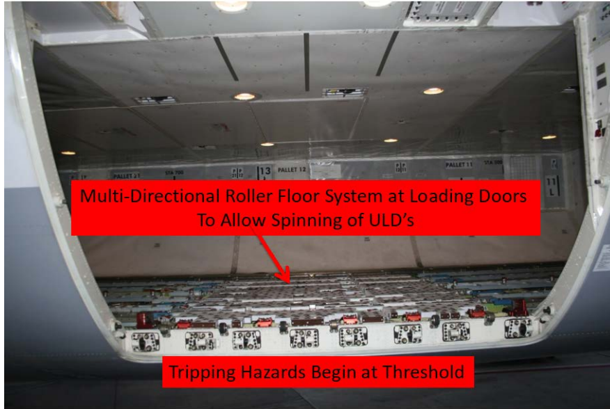
Figure 151. Cargo Door Opening—B-747-8I (Photograph courtesy of FAA)
