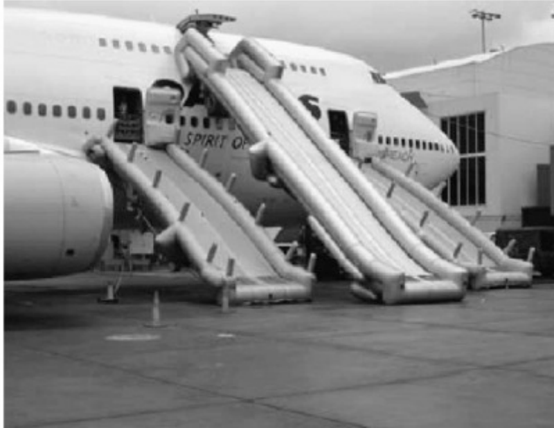
Figure 15. Slide Emergency Evacuation of a B-747-438—View 1 (Photograph courtesy of Australian Transport Safety Bureau)
