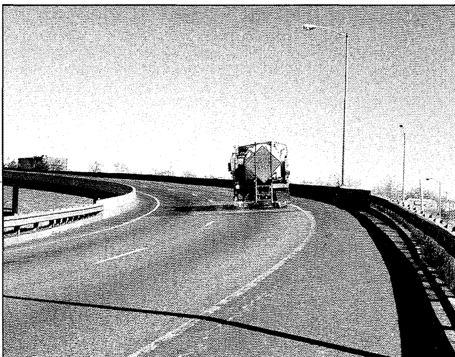
The Snow and Ice List Serve provides the latest in snow and ice control methods, such as the anti-icing application shown here.
