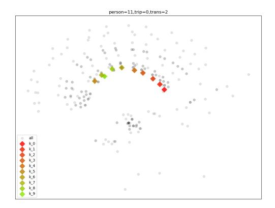
Figure 2 Person 11 Trip 1 requires 2 transfers to complete but the search space is very large. The MDS of the LCSWT distance matrix shows clear clusters of similar options in a fan like position at the top. The k-paths that are selected closely align to 10 of the 15 naturally occurring clusters.
