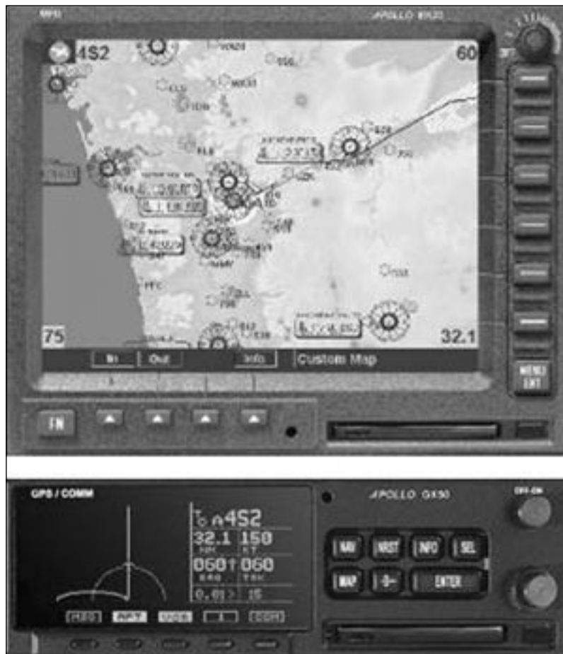
Figure 1. Capstone Avionics displays. The MX-20 display is shown on top, and the GX-60 GPS unit is shown below it.
