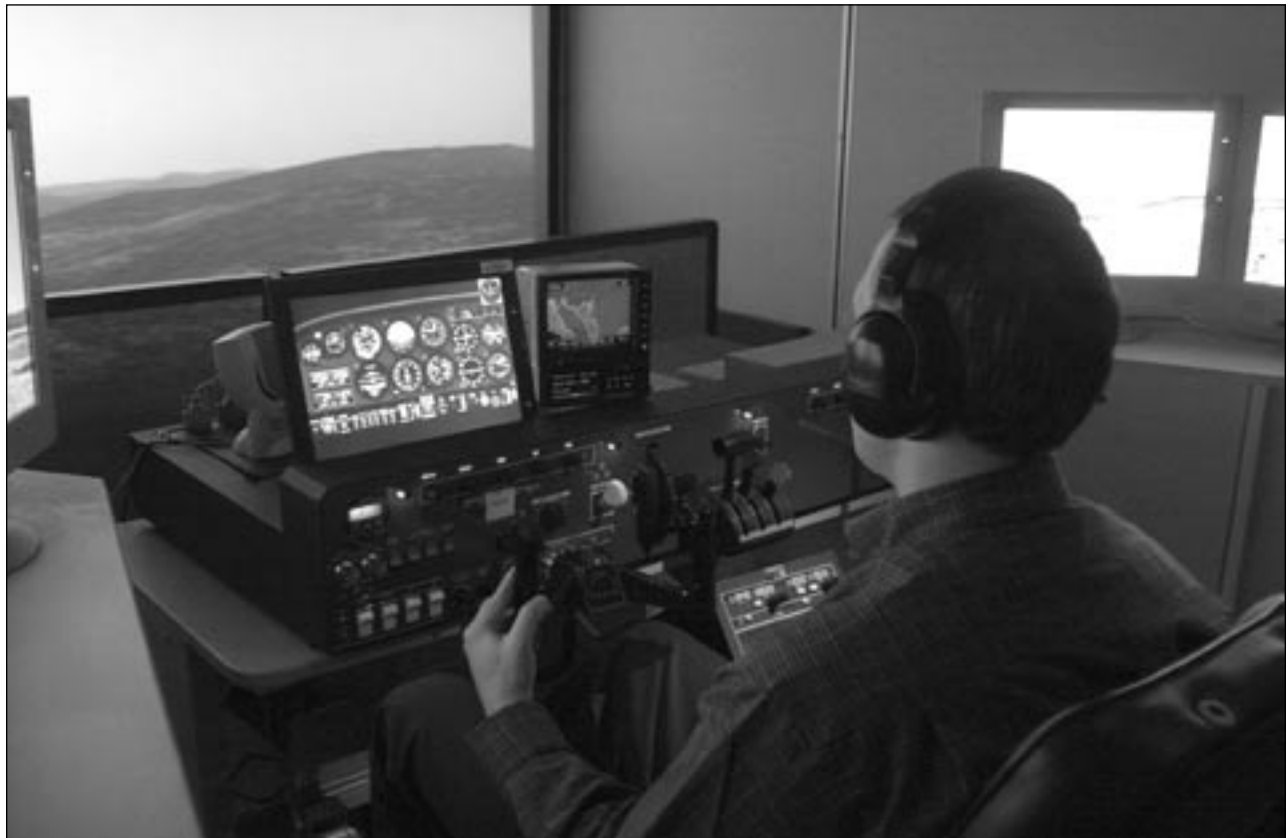
Figure 2. Basic General Aviation Research Simulator (BGARS).
