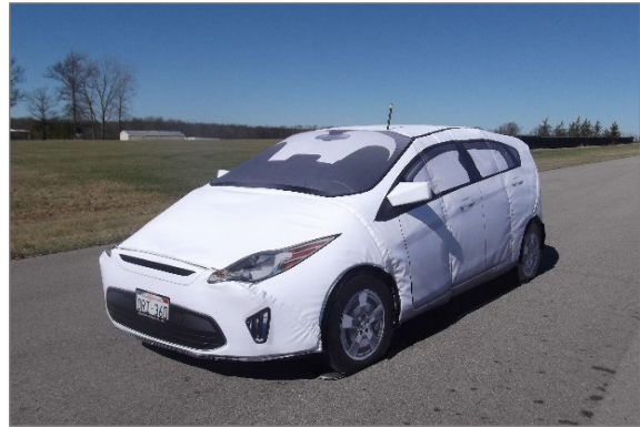
Figure 2-5. GVT atop of the LPRV
