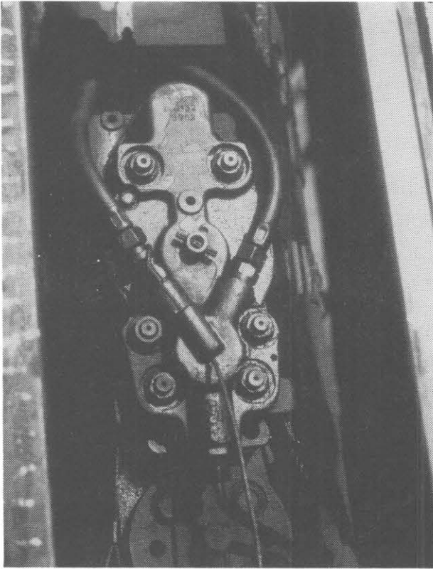
Figure 24.8 Fixed Four Step Fuel Pump on Delmag Hammer
