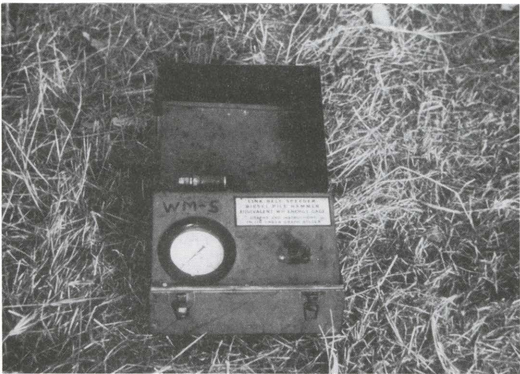
Figure 24.12 Typical External Bounce Chamber Pressure Gauge
