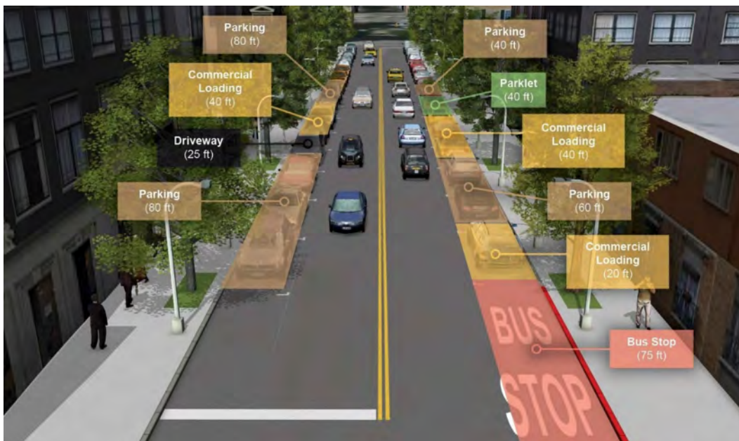
Figure 20. Graphic. An example of quantitatively visualizing the inventory of various curb uses on a typical block in San Francisco, CA, USA. Source: Fehr & Peers/Uber Technologies.
