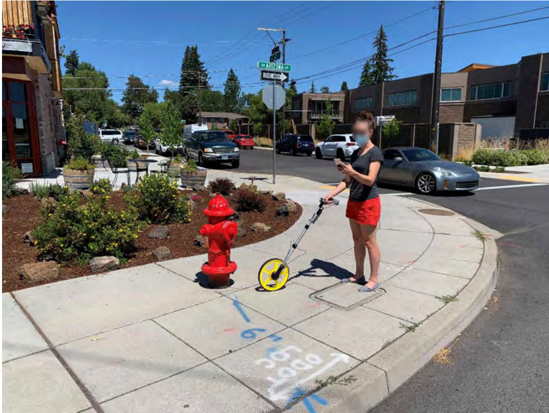
Figure 26. Photo. Surveyor uses CurbWheel and smartphone app to inventory curbside assets and regulations. Source: SharedStreets.
