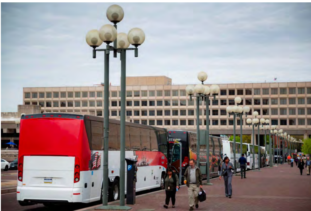
Figure 41. Photo. In contrast, the provision of ample first-in/first-out curb loading space allows safe and orderly access for tour buses elsewhere in Washington, DC, USA. Source: District Department of Transportation.
