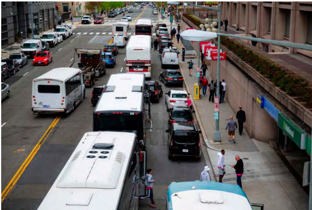
Figure 40. Photo. Lack of curb loading space in high-demand areas results in lane blockages and undesirable vehicle movements resulting from tour bus pick-up/drop-off activity in Washington, DC, USA. Source: District Department of Transportation.
