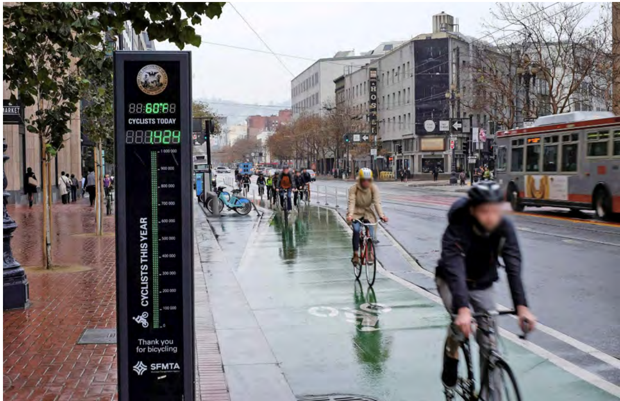
Figure 45. Photo. Curbside bicycle counting sensor and digital sign installed to inventory use of curbside bicycle facility in San Francisco, California, USA.
