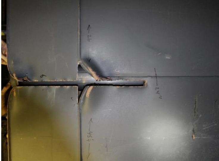
Figure 38. Tear in Test 1 Fuel Tank
