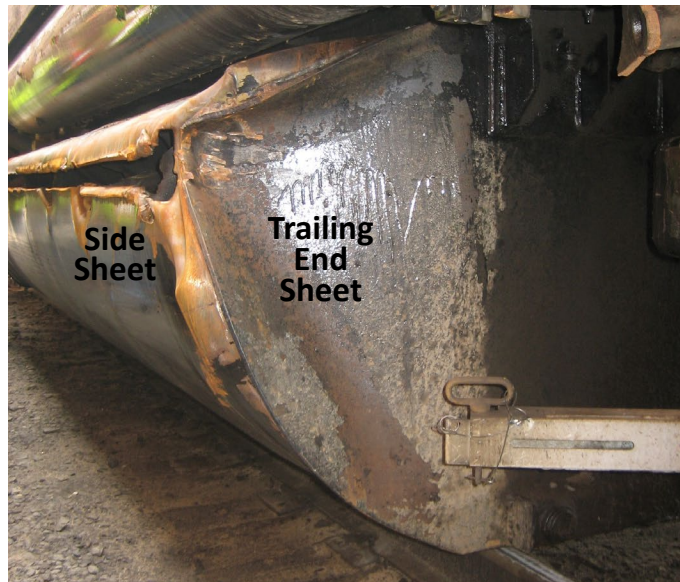
Figure 3. Damage to Lead Locomotive Fuel Tank
