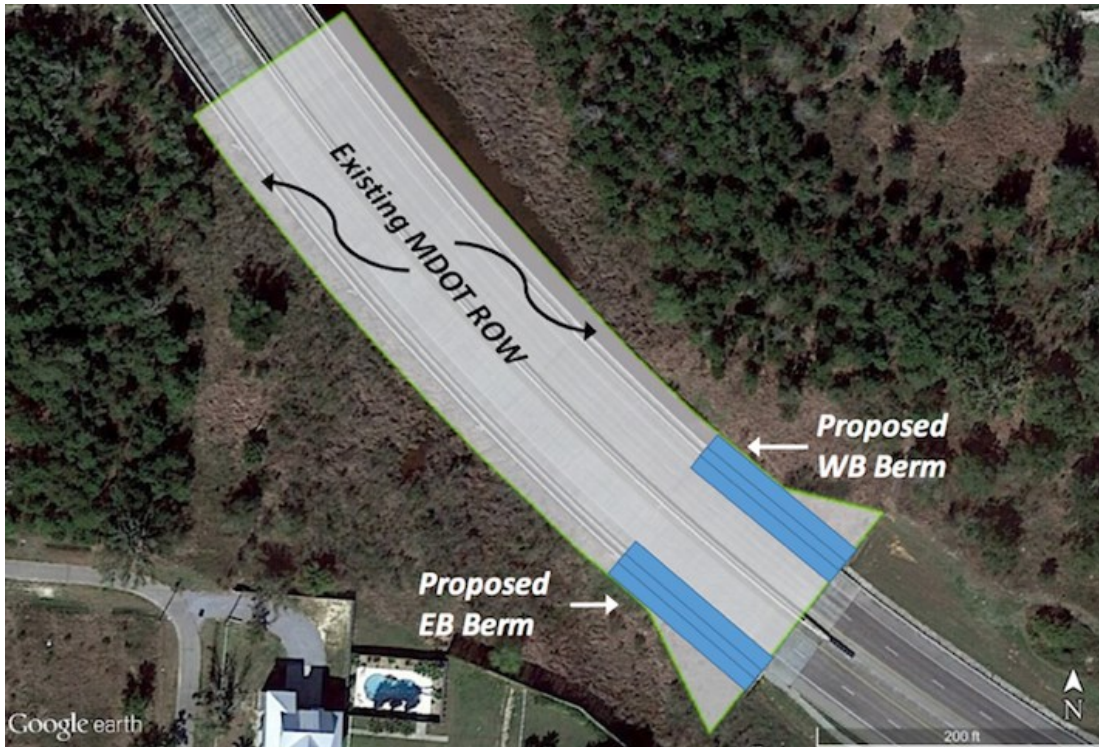
ES 1. General location overview showing the existing MDOT right-of-way and proposed westbound (WB) and eastbound (EB) berm locations relative to the bridge approach and bridge spans. (Map Credit: Google Earth; Map©2018Google)
