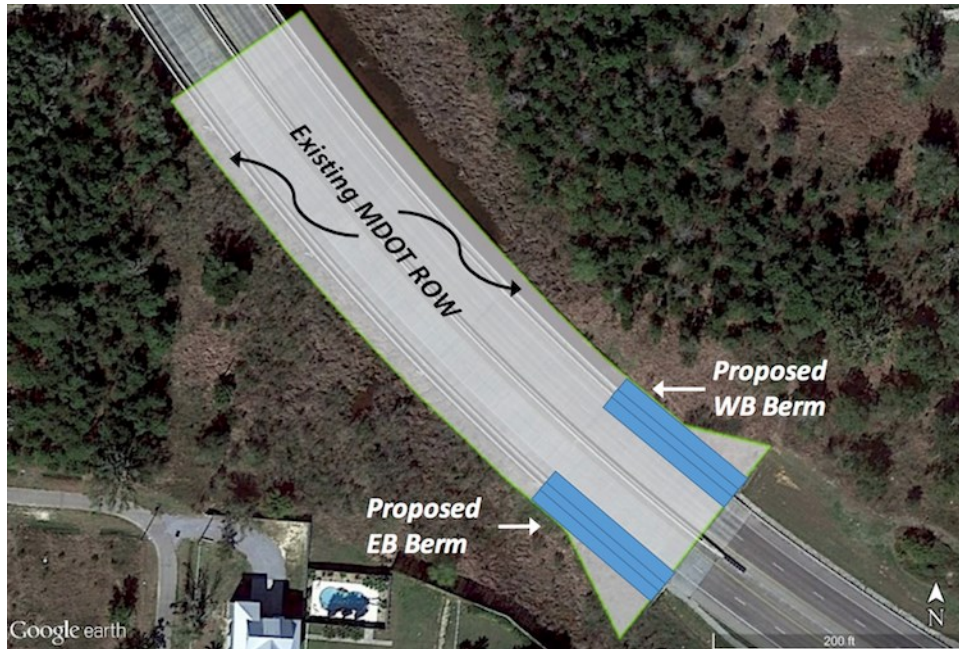
Figure 15. Overview image showing MDOTs existing right-of-way and the locations of the proposed berms adjacent to the lowest spans. (Photo credit: Google Earth; Map©2018Google)
