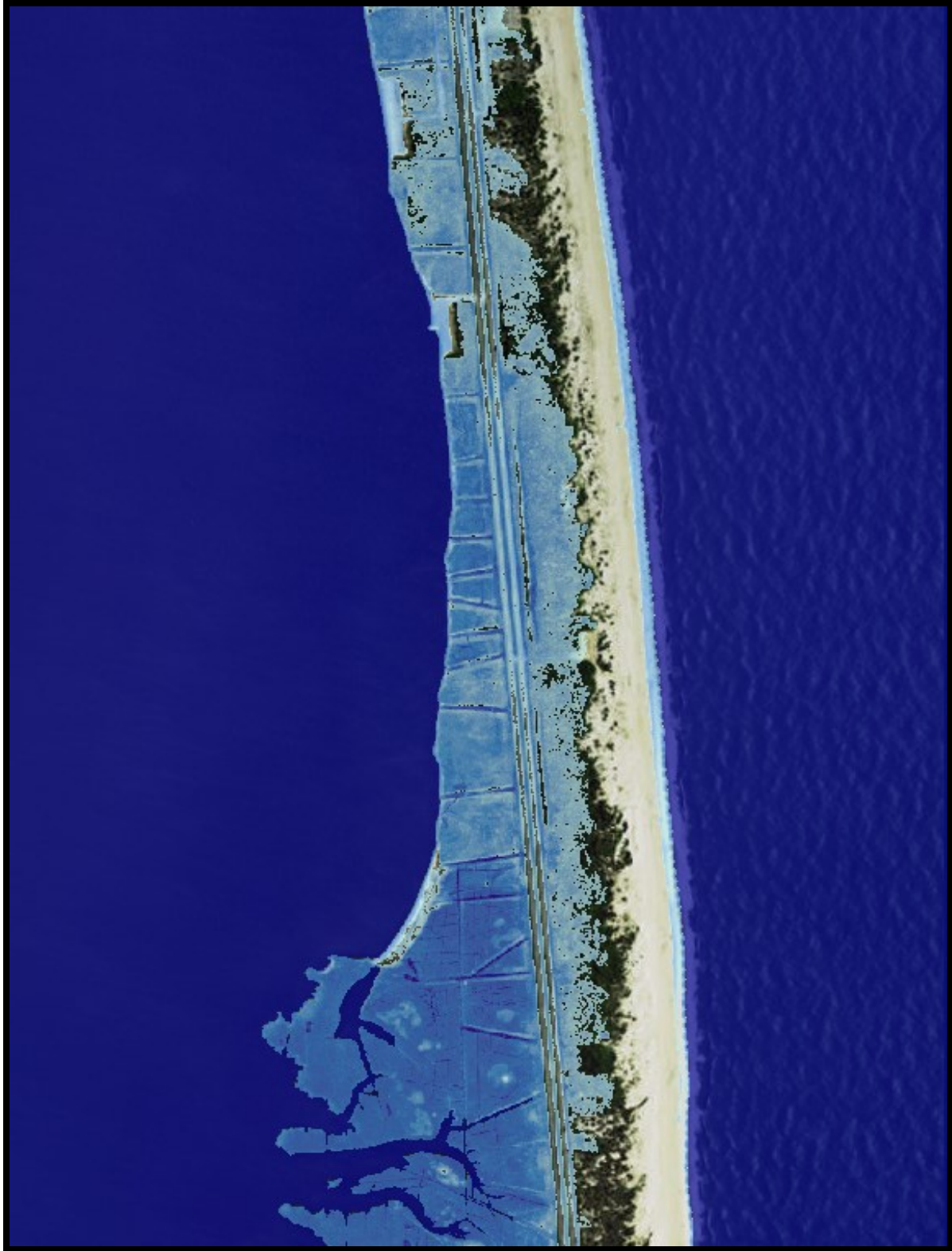
Figure 8 - Inundation along Middle Section of Study Area for 3 Feet (0.9 Meter) of Sea Level Rise (NOAA, 2017) – note that the area shaded light blue reflects inundated areas.
