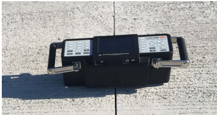
Figure 7. Photo. Transverse contraction joint activation testing with MIRA device.
