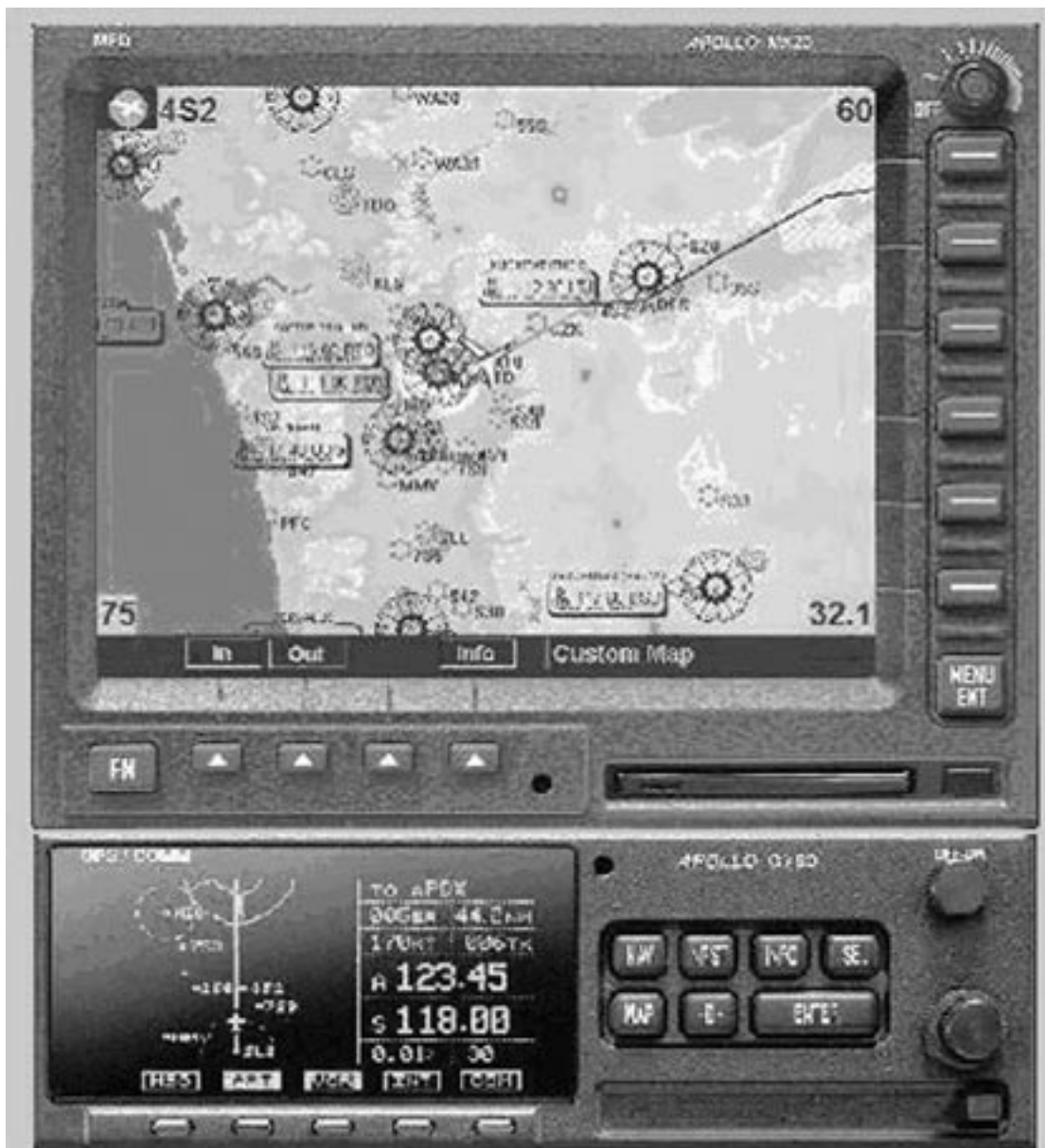
Figure 1: Capstone Avionics displays. The MX-20 display is shown on top and the GX-60 GPS unit is shown below it.
