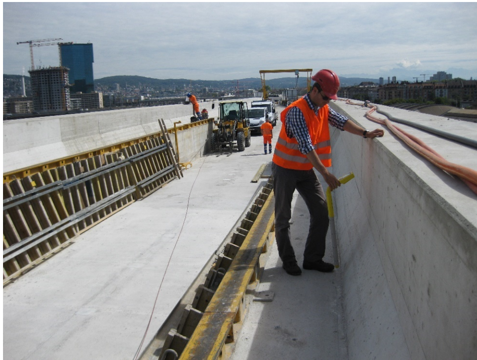
Figure 34. Photo. On-site detection of EIT breach on a post-tensioned structure.
