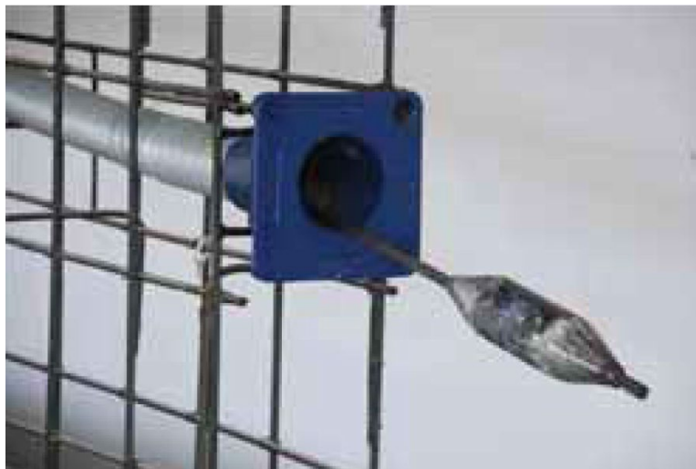
Figure 16. Photo. Plunger test to detect duct kinks, deformations, or obstructions.
