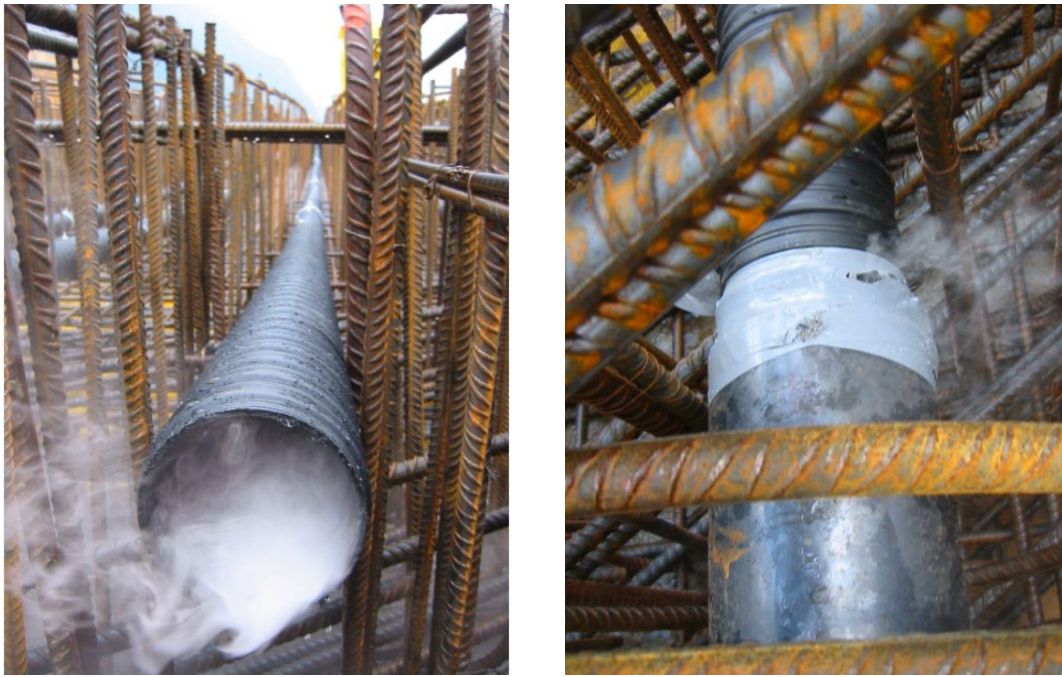
Figure 17. Photo. Dry ice (CO 2 ) fog test to detect leaks in duct.
