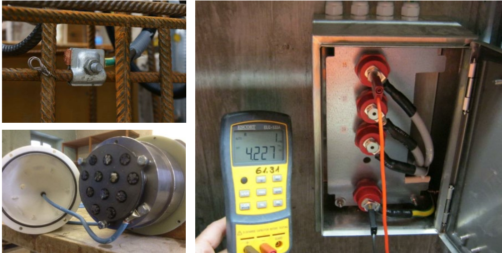
Figure 14. Photo. Wire conductors lead from mild reinforcement (top left) and strand anchor head (bottom left) to junction box where an LCR meter can be used to measure impedance (right).
