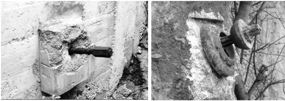
Figure 2. Photo. Examples of early ground anchorage tendon failures prior to development of EIT technology.
