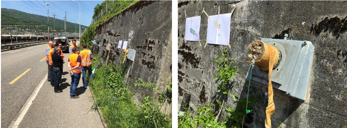
Figure 6. Photo. Overview of ground anchor wall (left) and close-up view of ground anchorage with end cap removed and lead wire clipped to a strand for electrical resistance measurement (right).
