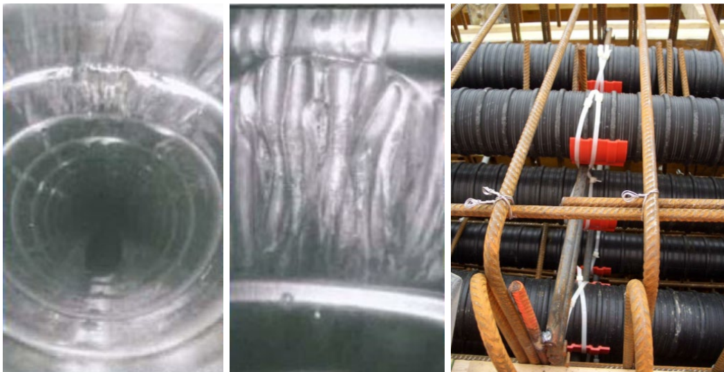
Figure 13. Photo. Abrasion of inside surface and potential breach of plastic ducts from pulling of strands around tight bends or local protrusions (left and center, courtesy of SBB) and protective half-shells at duct support points (right, Stahlton).
