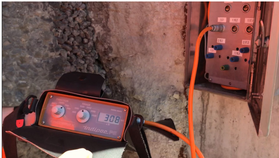
Figure 7. Photo. In-service measurement of anchor force by electrical load cells. The leads for the electrical resistance measurements on selected anchors are connected to the same junction box (blue plug sockets).
