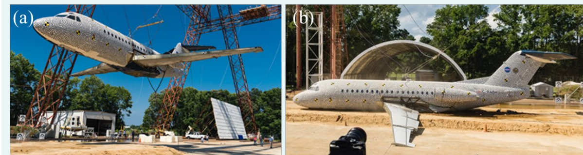
Figure 3. Full-scale drop test of a Fokker F28 aircraft (a) pre-test and (b) post-test
