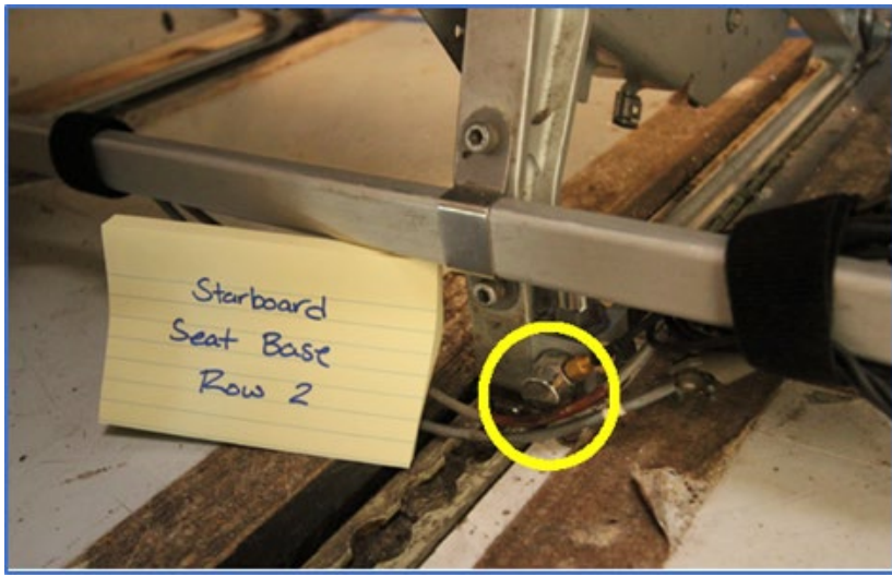
Figure 10. (a) Schematic of the F28 aircraft showing the location of a seat base accelerometer and (b) a photo of an actual seat base accelerometer
