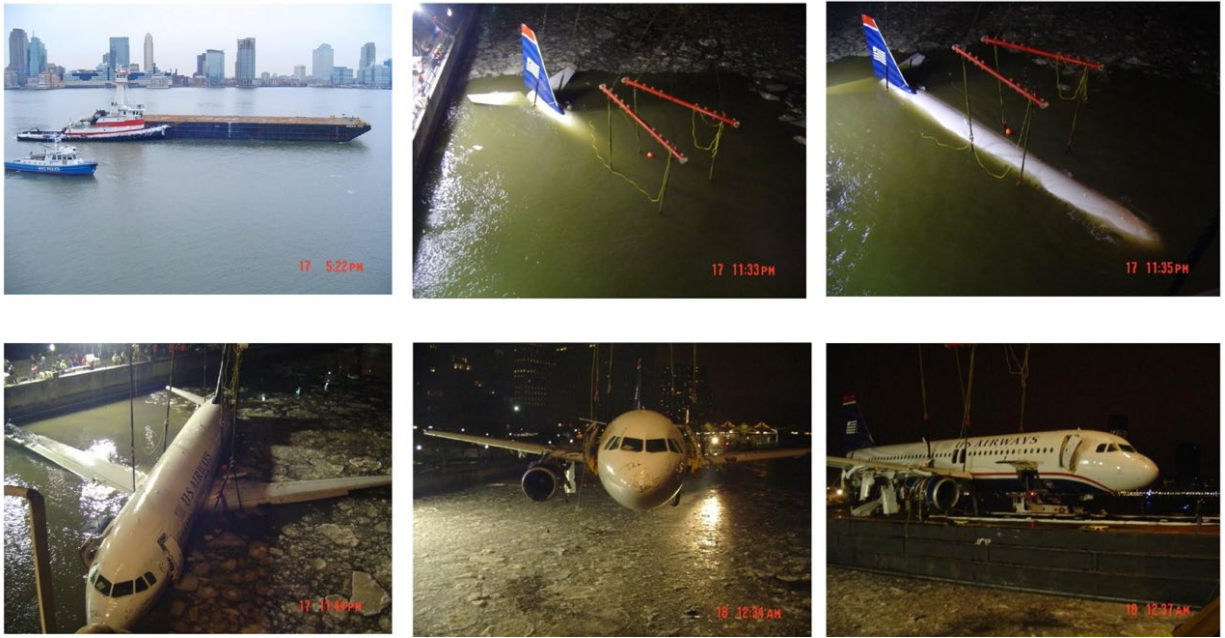
Figure 7. Montage of photographs of the A320 aircraft being recovered
