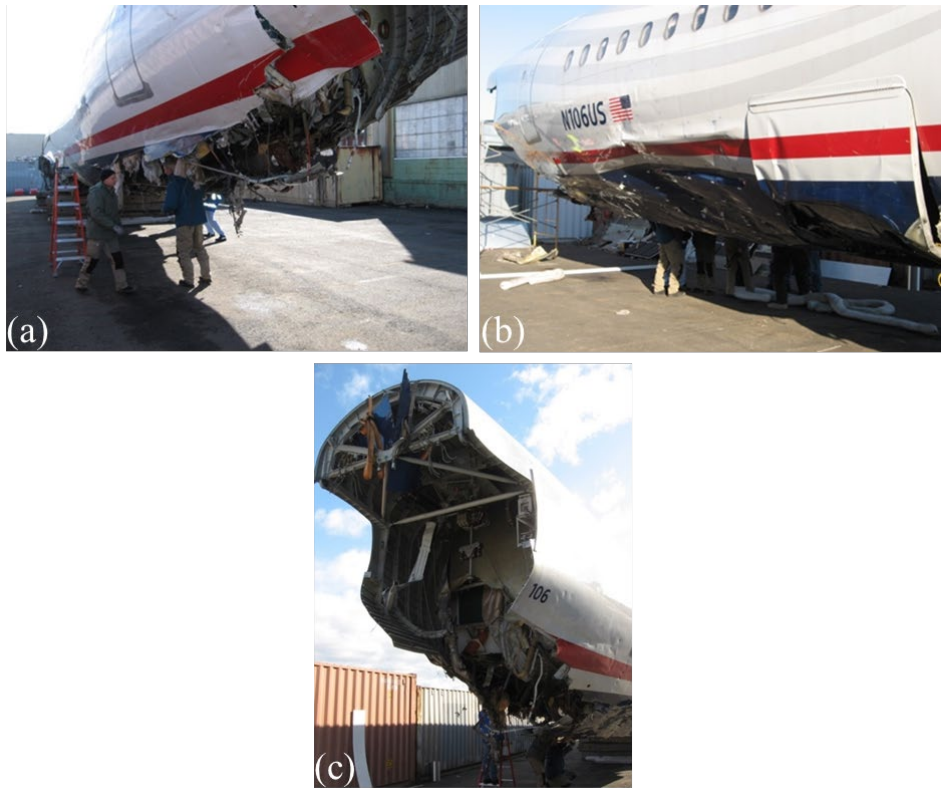
Figure 8. Damage to tail section looking (a) forward, (b) aft, (c) after removal of damaged parts
