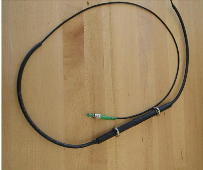
Figure B-7. Fiber optics strain gauge (FOSG)
