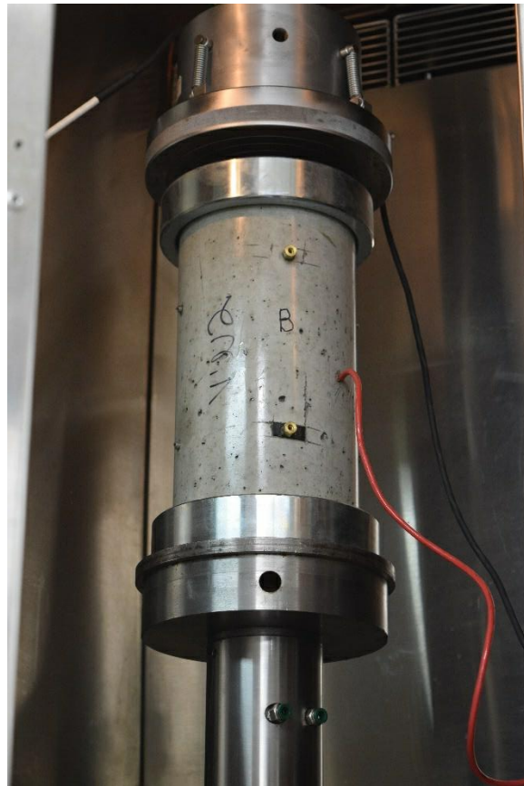
Figure B-10. Specimen setup in the MTS testing machine and environmental chamber
