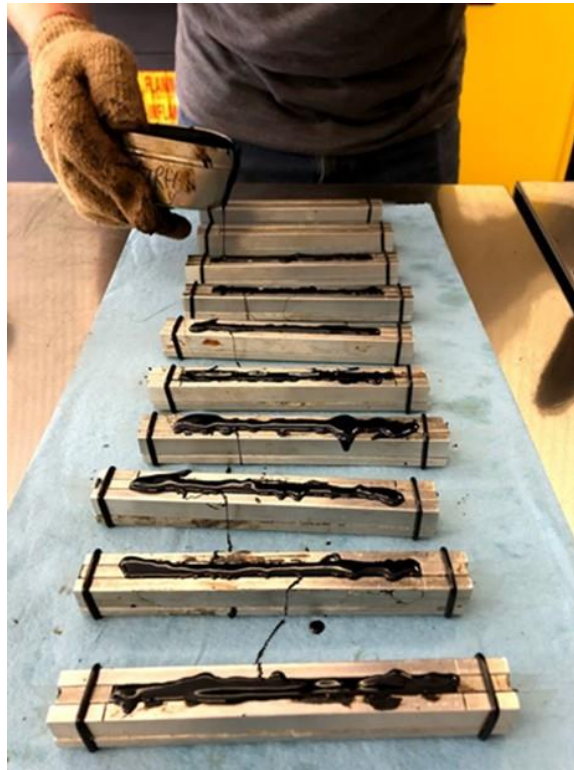
Figure 17. Photo. Pouring asphalt binder into molds.
