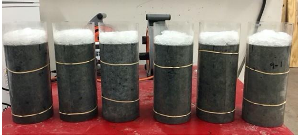
Figure 12. Photo. Snow melting test setup with plastic sheets wrapped around cylinders (after 1 hour).
