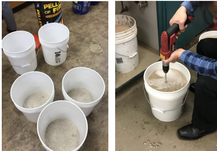
(a) Proportioning (left) and mixing in warm water (right)
