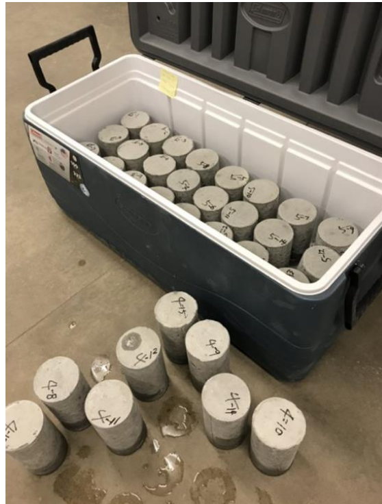
Figure 34. Photo. Four-inch-diameter concrete cylinders in moisture curing box.
