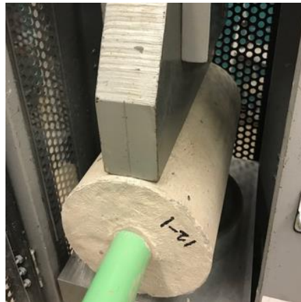
Figure 49. Photo. Removal of concrete from corrosion sample.
