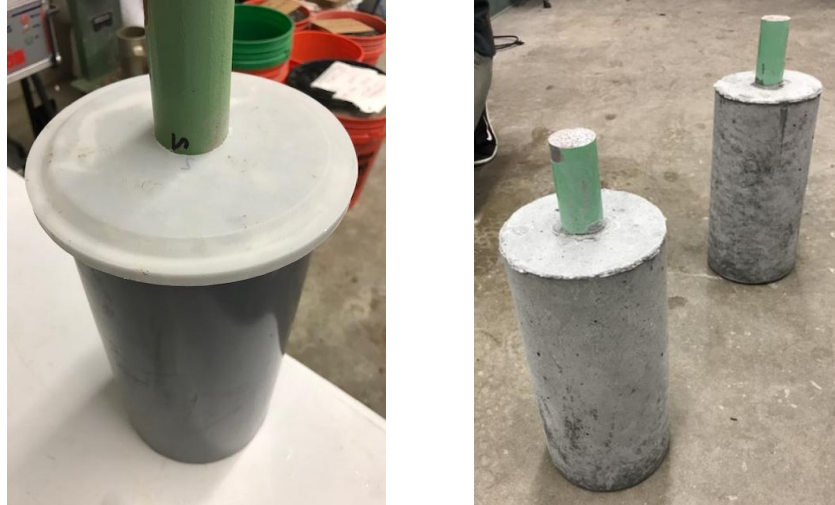
Figure 36. Photos. Plastic mold (left) for 6×12-inch cylinders with dowel bars (right).
