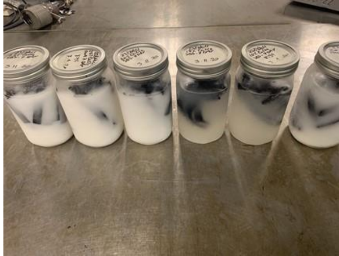
Figure 18. Photo. Asphalt binder beams soaking in jars with different brines.
