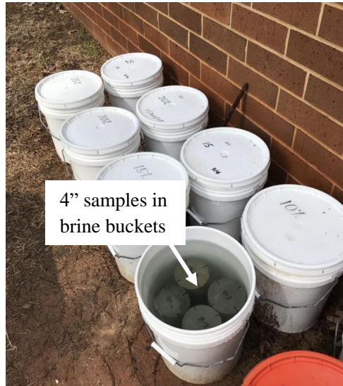
Figure 38. Photo. Ambient erosion test setup.
