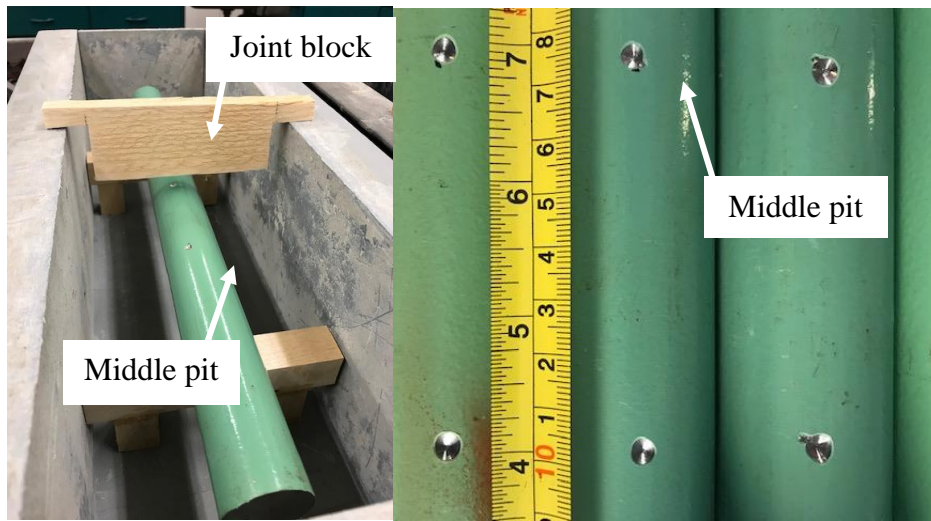
Figure 51. Photo. Plastic mold for joint samples with wood chairs (left) and dowel bars with pits (right).
