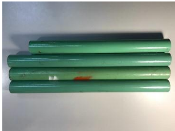
Figure 35. Photo. EC dowel bars for corrosion test.
