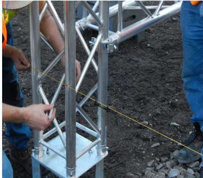
Figure 4. Camera Height Set a Known Distance above the Rail
