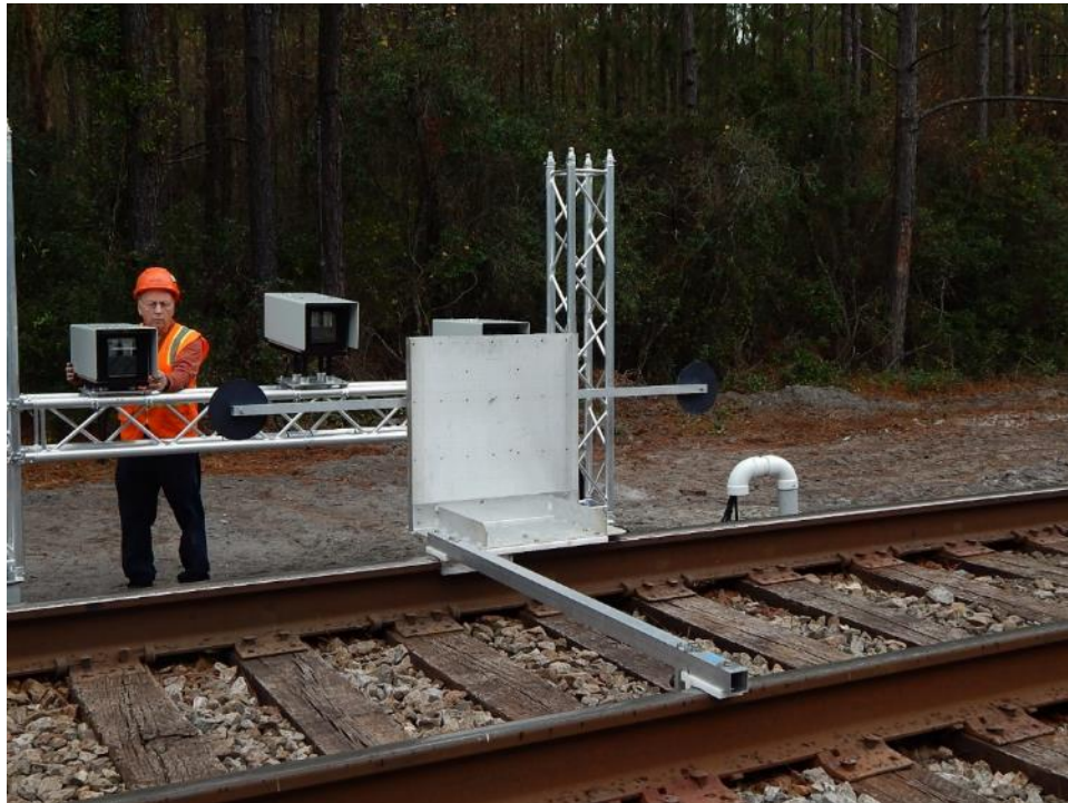
Figure 11. Cameras Adjusted to Align the Image in the Camera Field of View
