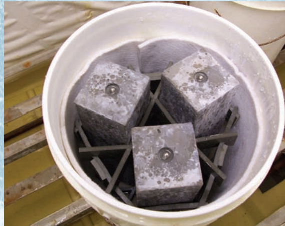
ASTM C 1293 samples (CANMET Laboratory, Canada) (Image submitted by Bebe Resendez, Transtec Group)
