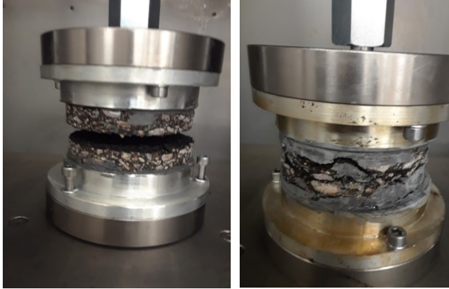
Figure 16. Testing for bond surface energy in an asphalt mixture performance tester (AMPT): control sample with a normal bonding material (left) and sample containing VRAM layer (right)
