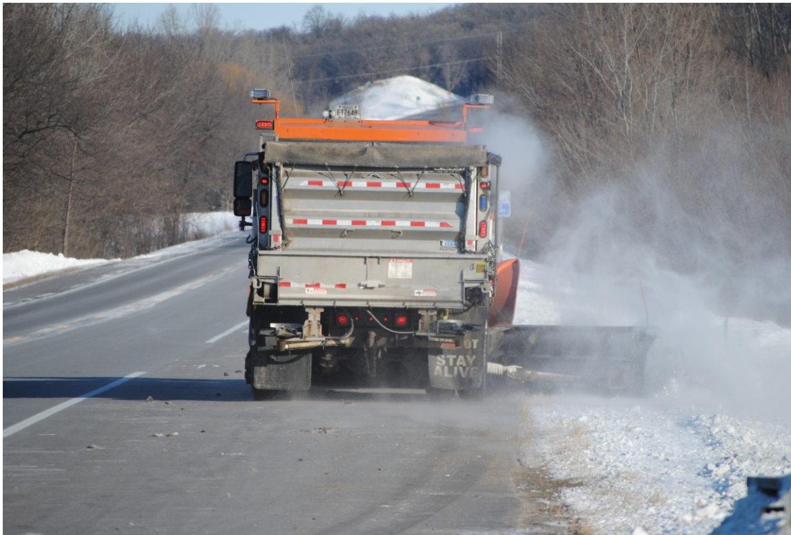
Figure 2: Winging the roadway shoulder to improve safety and prepare for additional snow storage of future storm events.
