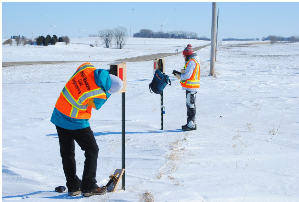
Figure 4: Time lapse camera being switched out for one with fresh batteries (left), and Kestrel and Hobo instruments being downloaded using iPad for communication (right). Ivanhoe location.
