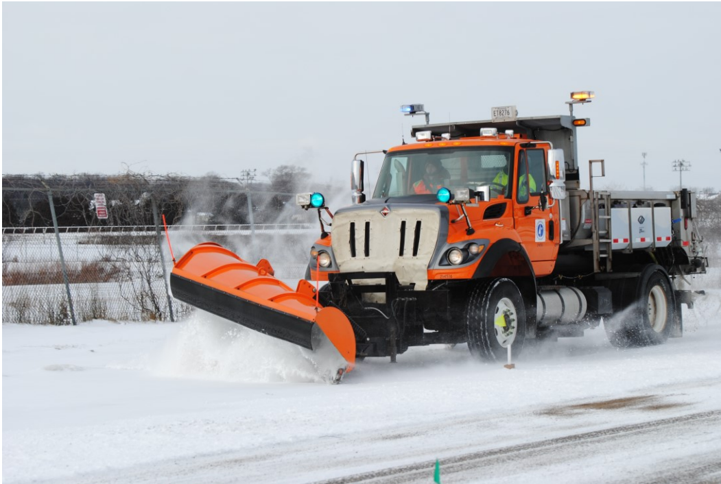
Figure 1: Typical MndOT winter maintenance truck, circa 2016, outfitted with front, right wing and underbody plows, brine saddle tanks and rear deicer distribution system.
