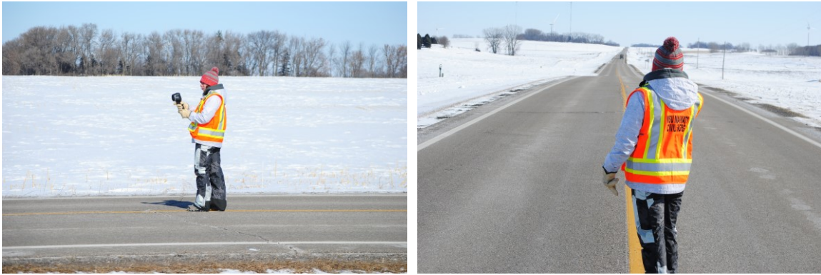
Figure 5: Measurement of roadway temperatures using FLIR E6.
