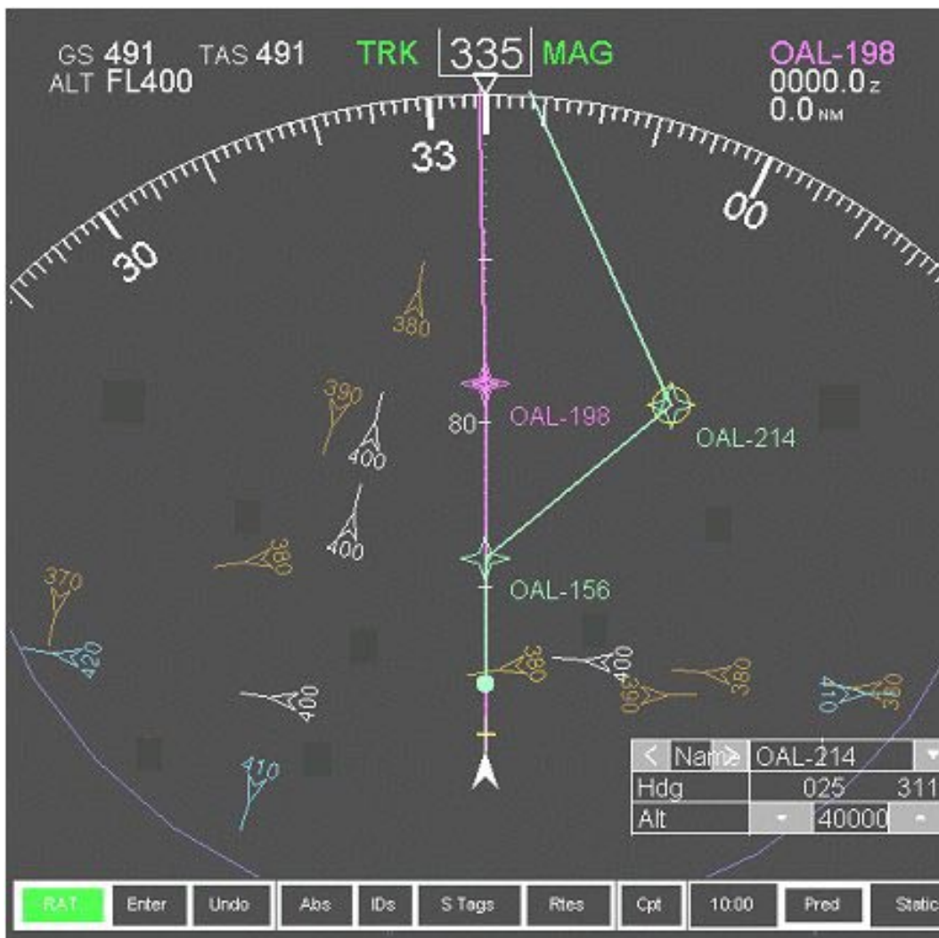
Figure A10. The CDTI as it appears when changes to planned heading are assessed.
