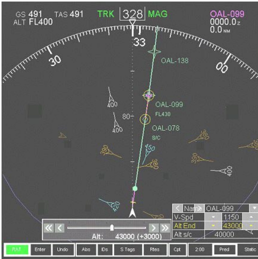
Figure A7. The CDTI as it appears when a new value for altitude is proposed.
