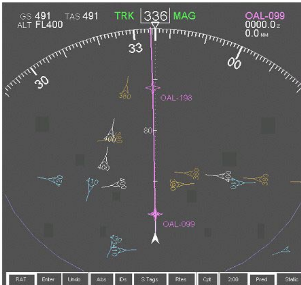
Figure 2. The version of NASA's CDTI that was used in the current analysis.
