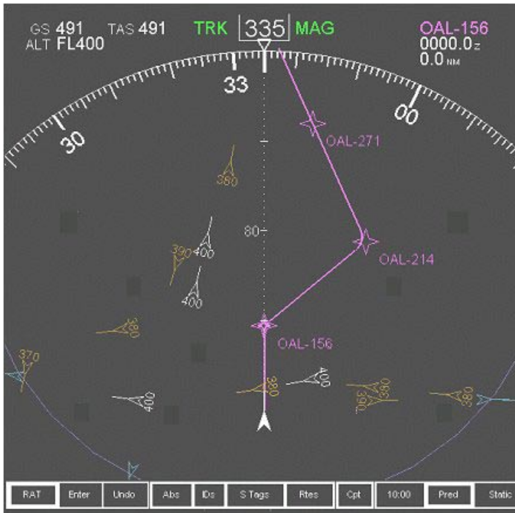
Figure A11. The CDTI as it appears when changes to heading have been accepted.
