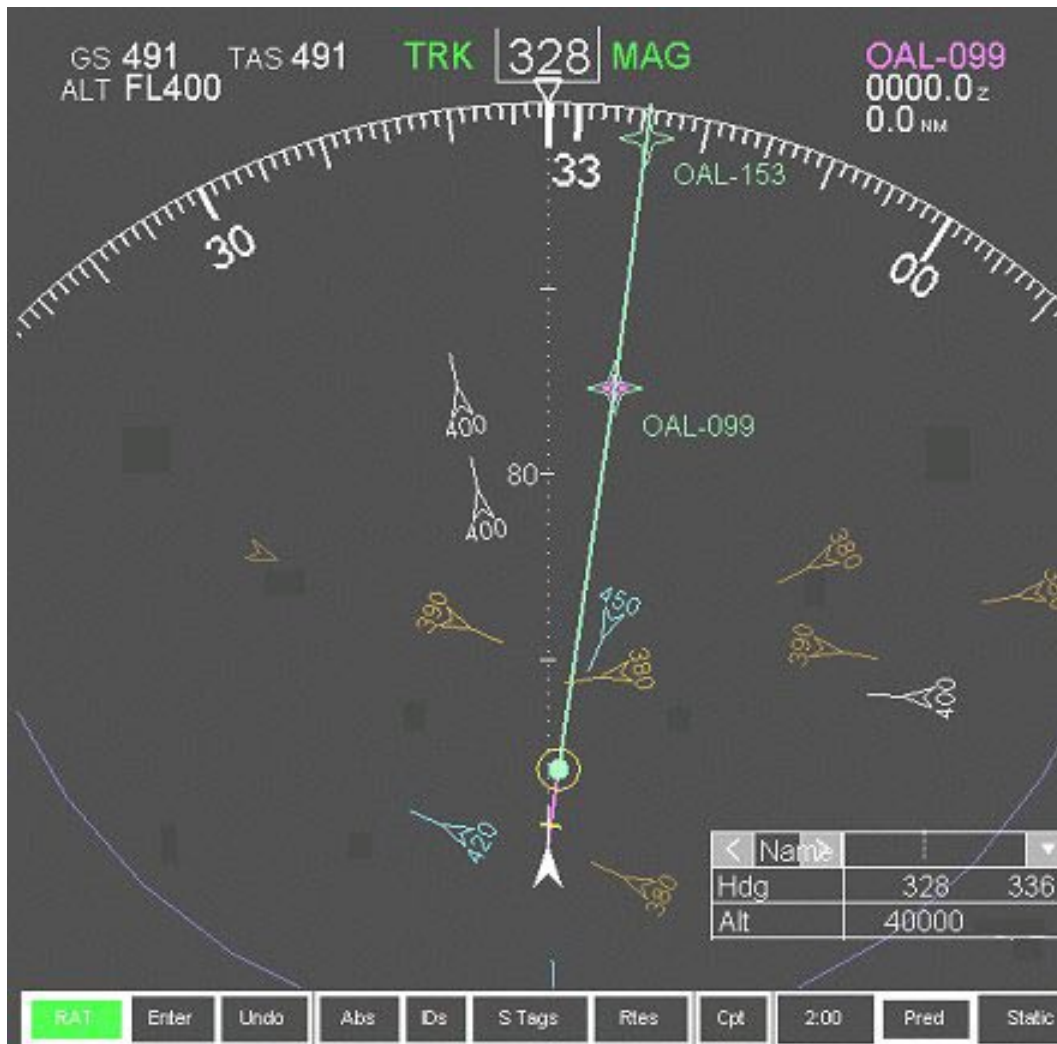
Figure A4. NASA's CDTI with the RAT tool and its respective window activated point" is selected.
