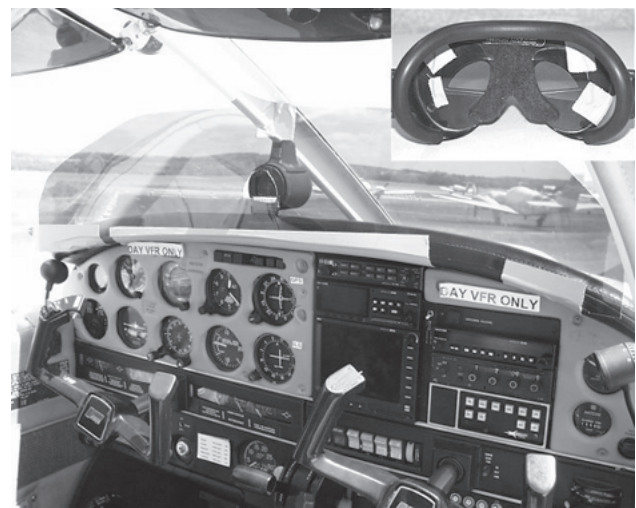
Figure 3. Polaroid material across windscreen of Piper Archer with (inset) Francis hood.
