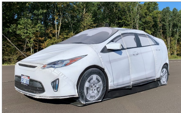
Figure 2-3. GST system, shown with GVT revision F
