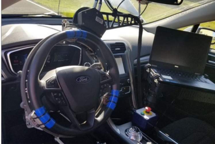
Figure 2-8. Example robotic steering controller installation
