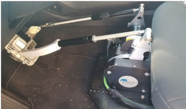
Figure 2-9. Example robotic brake and accelerator controller installation used in SV and LV
