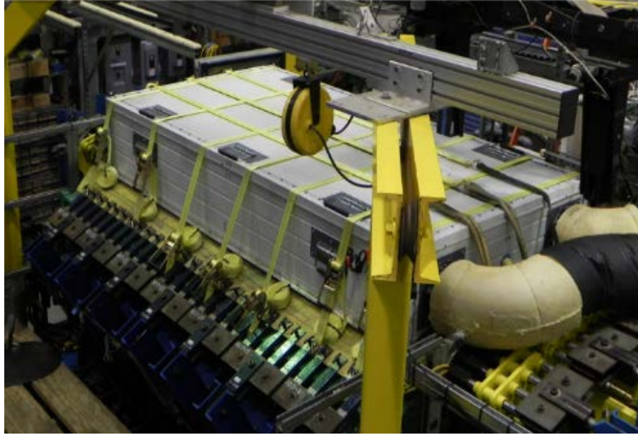
Figure A-6. Environmental chamber strapped to fuselage panel
