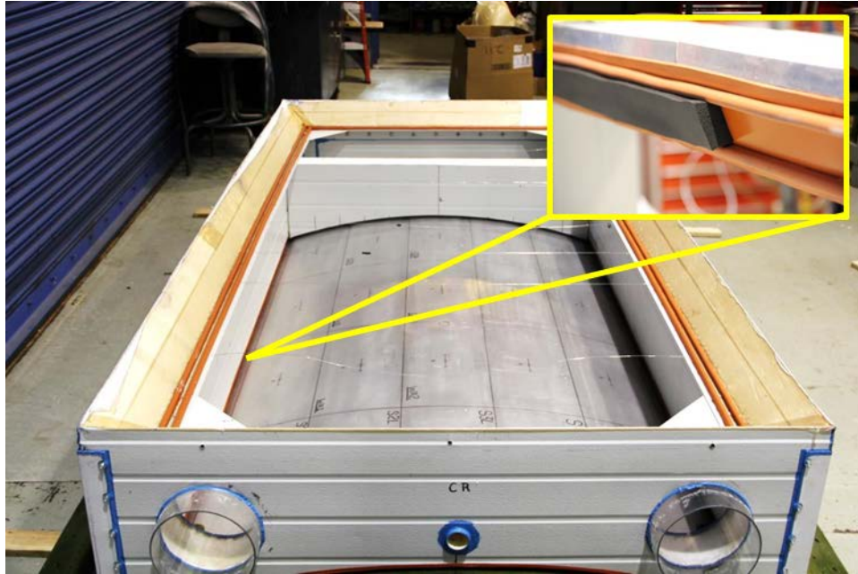
Figure A-3. Environmental chamber with airtight seal; insert shows the bottom seal consisting of rubber bulb seal and weather-resistant neoprene foam
