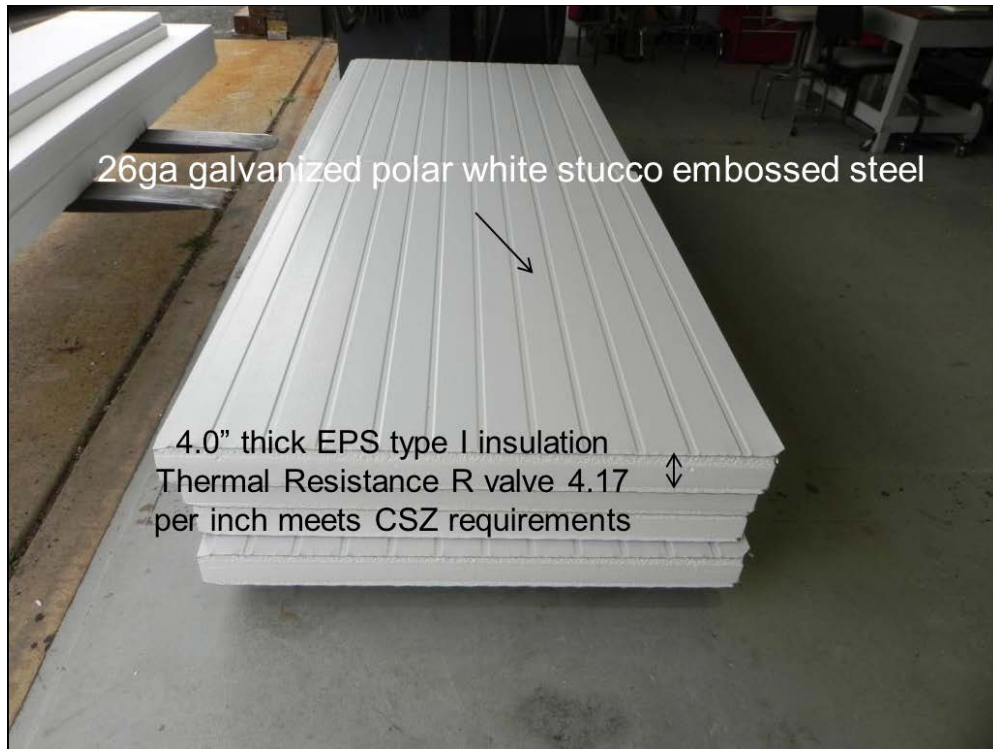
Figure A-4. Insulation material for environmental chamber
