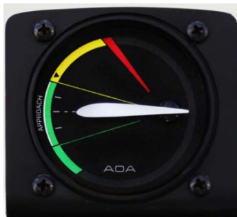
Figure 5. Dial AOA indicator with color coding [5]
