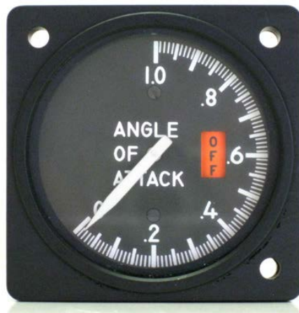
Figure 4. Dial AOA indicator with normalized scale [5]
